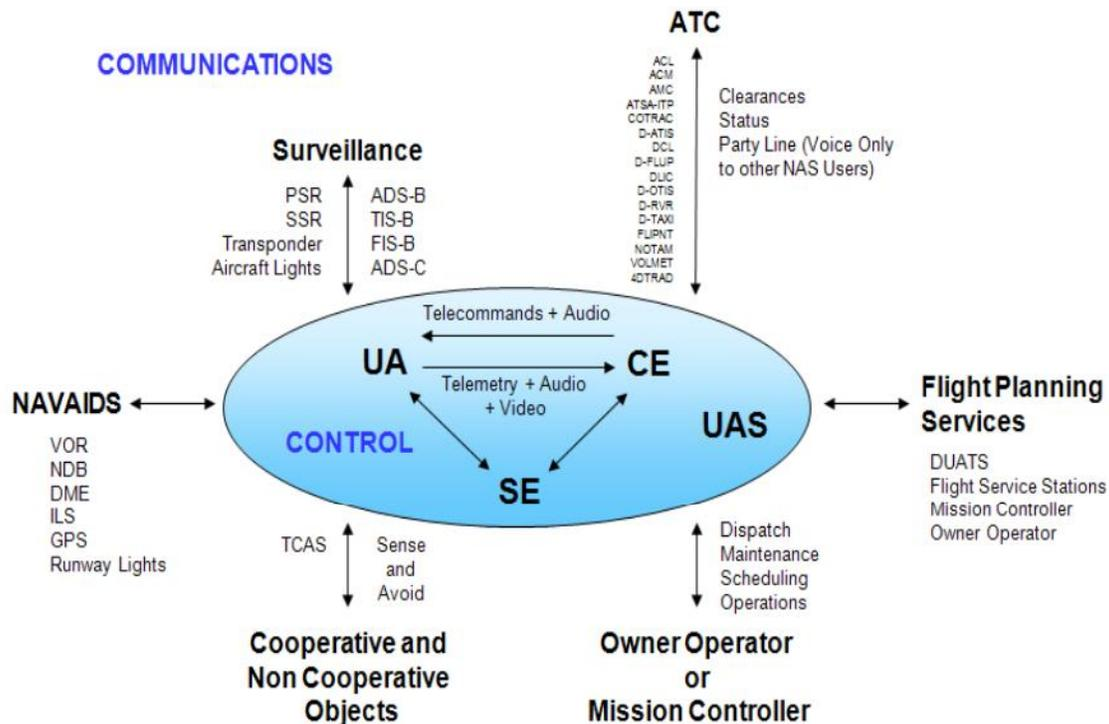
Figure 1 - Communications Interfaces for UAS Operations [RTCA SC-203]
