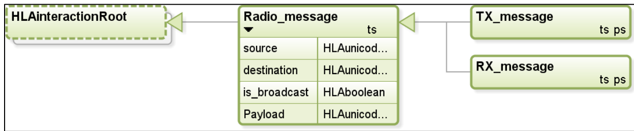
Figure 5. Radio message object model template
