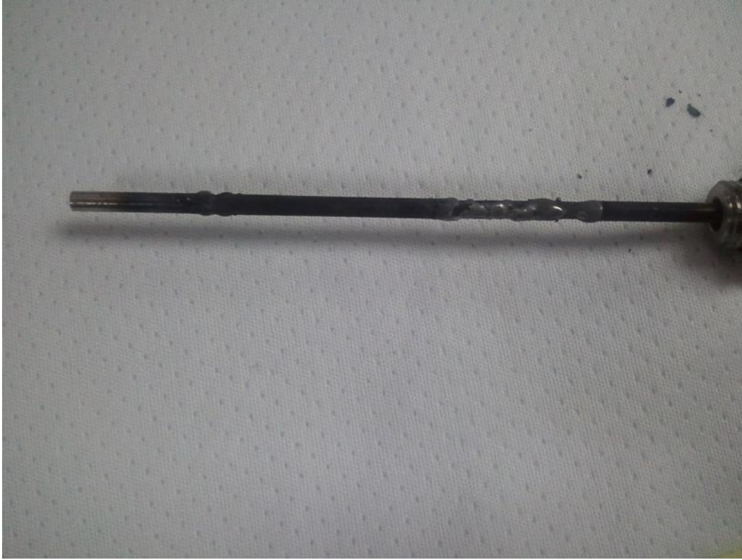
Figure D.37.—Fluid immersed portion of Heater 1: Note two melted areas.
