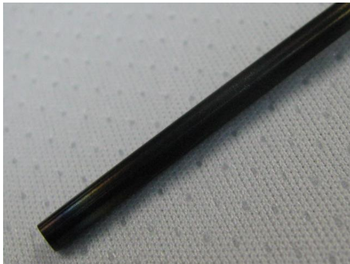
Figure D.64.—Heater 2 fluid immersed portion: Note bluing and blackening.
