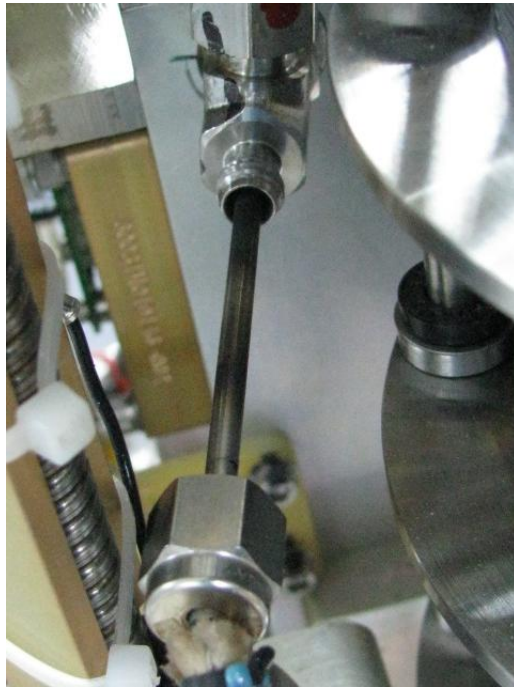
Figure D.13.—Heater 1 extracted from tee to maximum possible extent.
