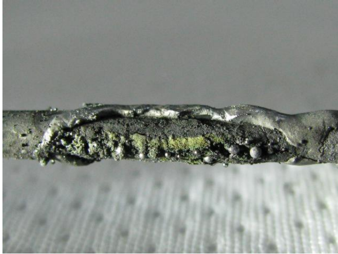
Figure D.25.—Close-up of Heater 1 melted surface.
