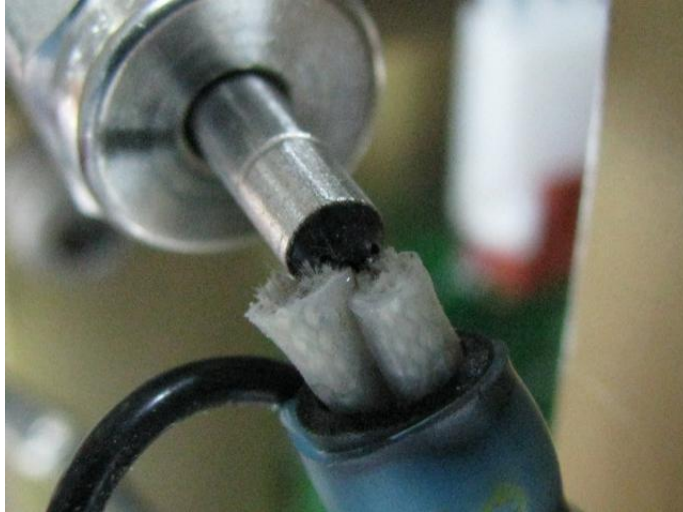
Figure D.57.—Heater 2 connection into TC.
