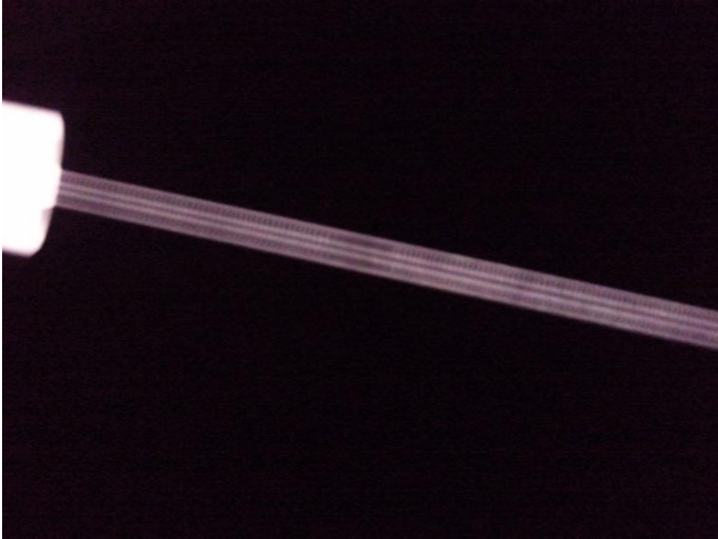
Figure E.76.—Close-up of heating element for Bulk Fluid Heater 3. Note irregularities.
