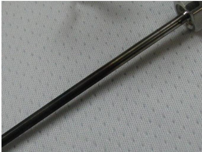
Figure D.67.—Heater 2 fluid immersed portion: Note blackening.
