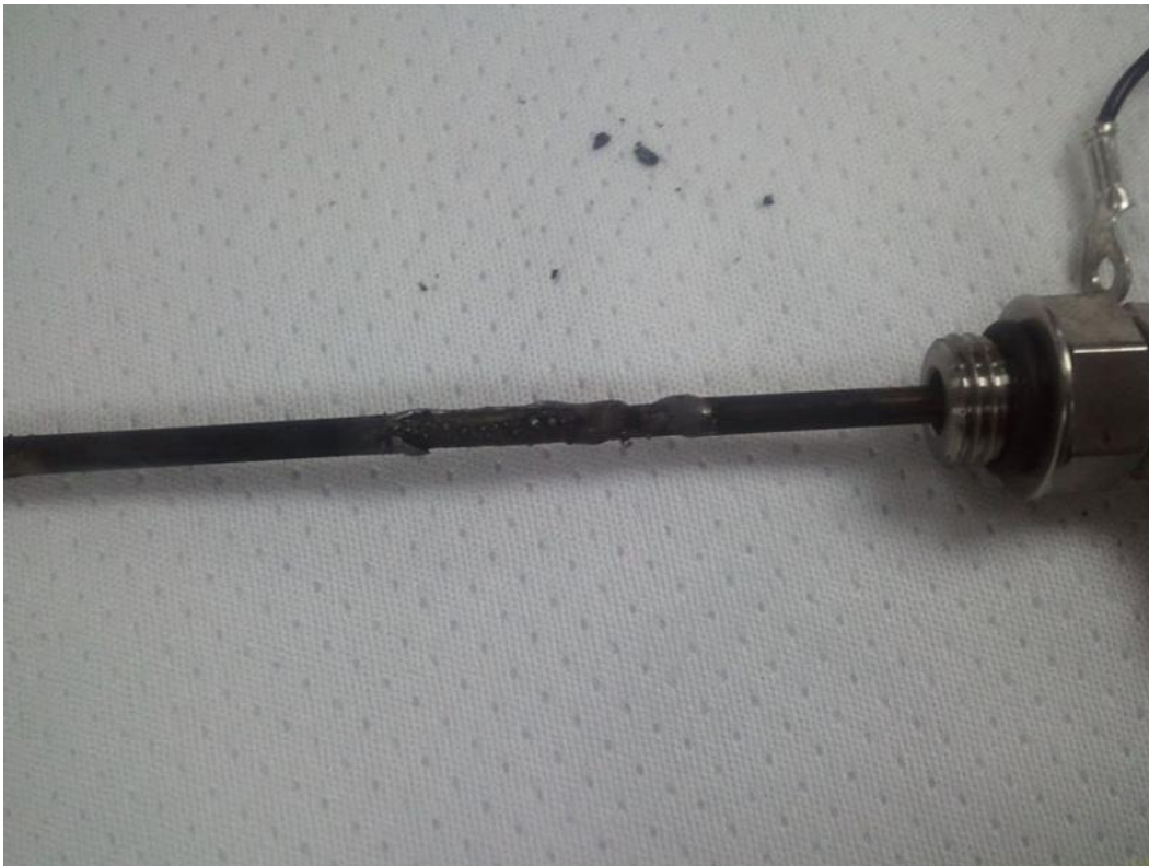
Figure D.44.— Heater 1: Note melted area
