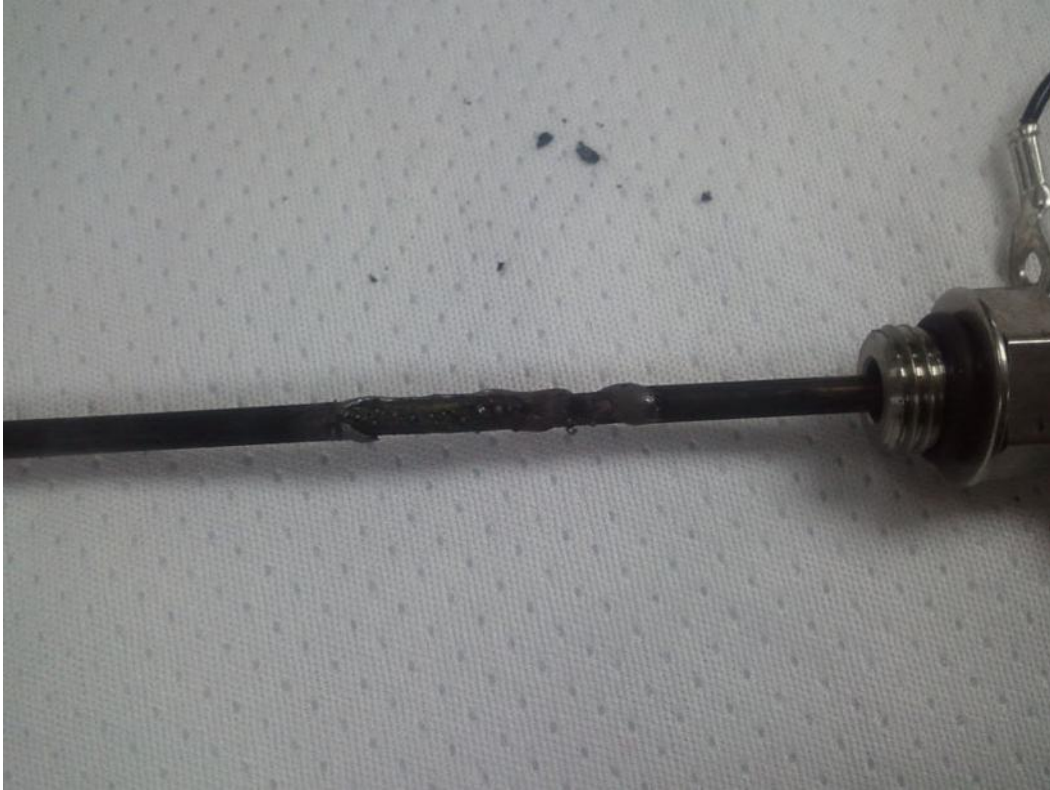
Figure D.43.—Heater 1: Note melted area.
