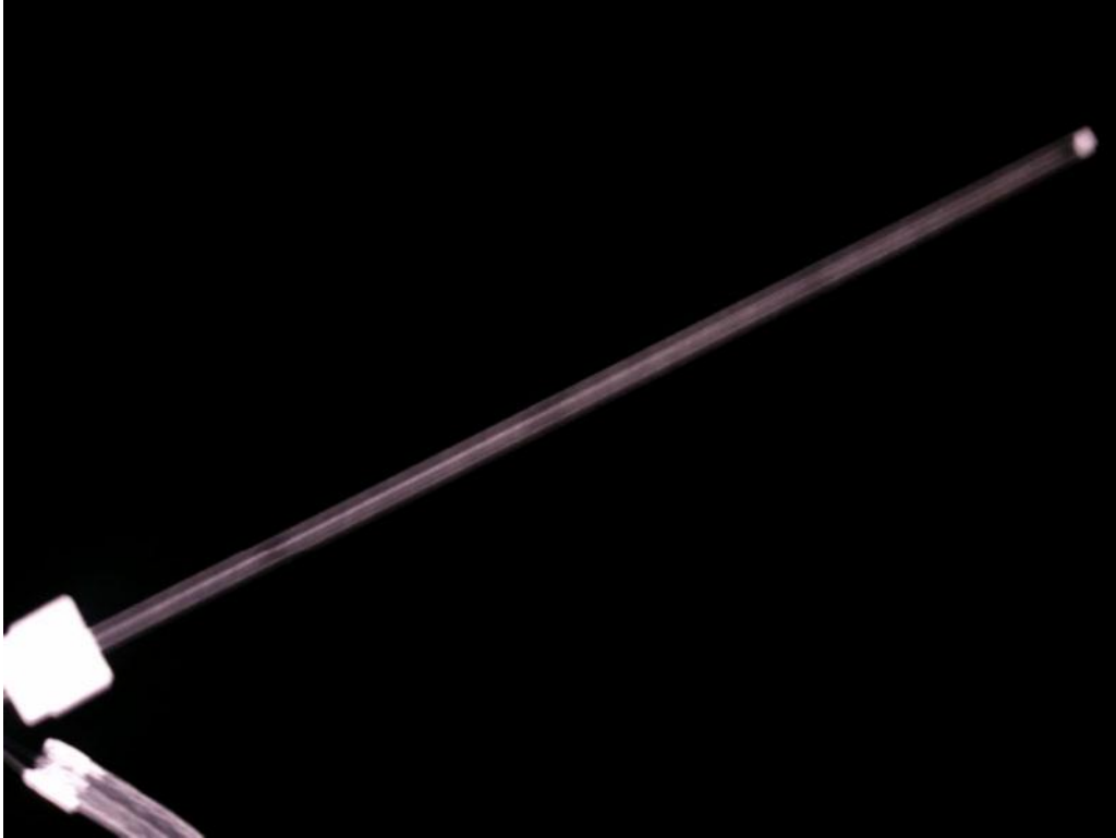
Figure E.48.—Heating element for Bulk Fluid Heater 2.
