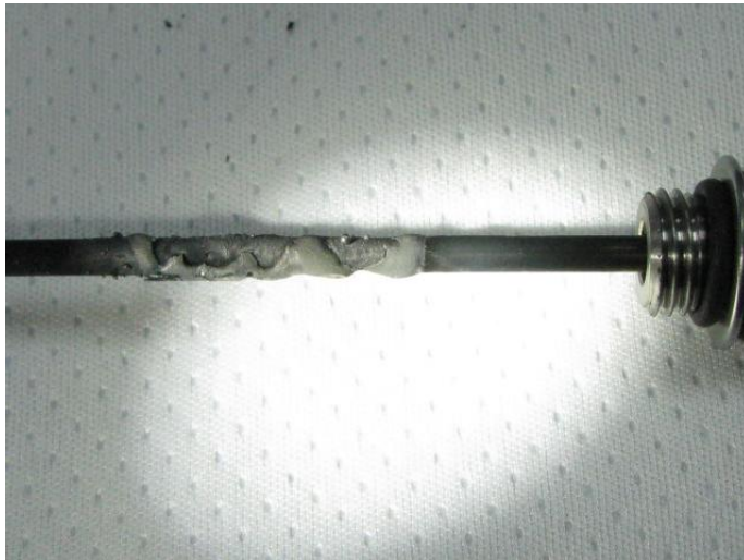
Figure D.29.—Heater 1 melted surface.
