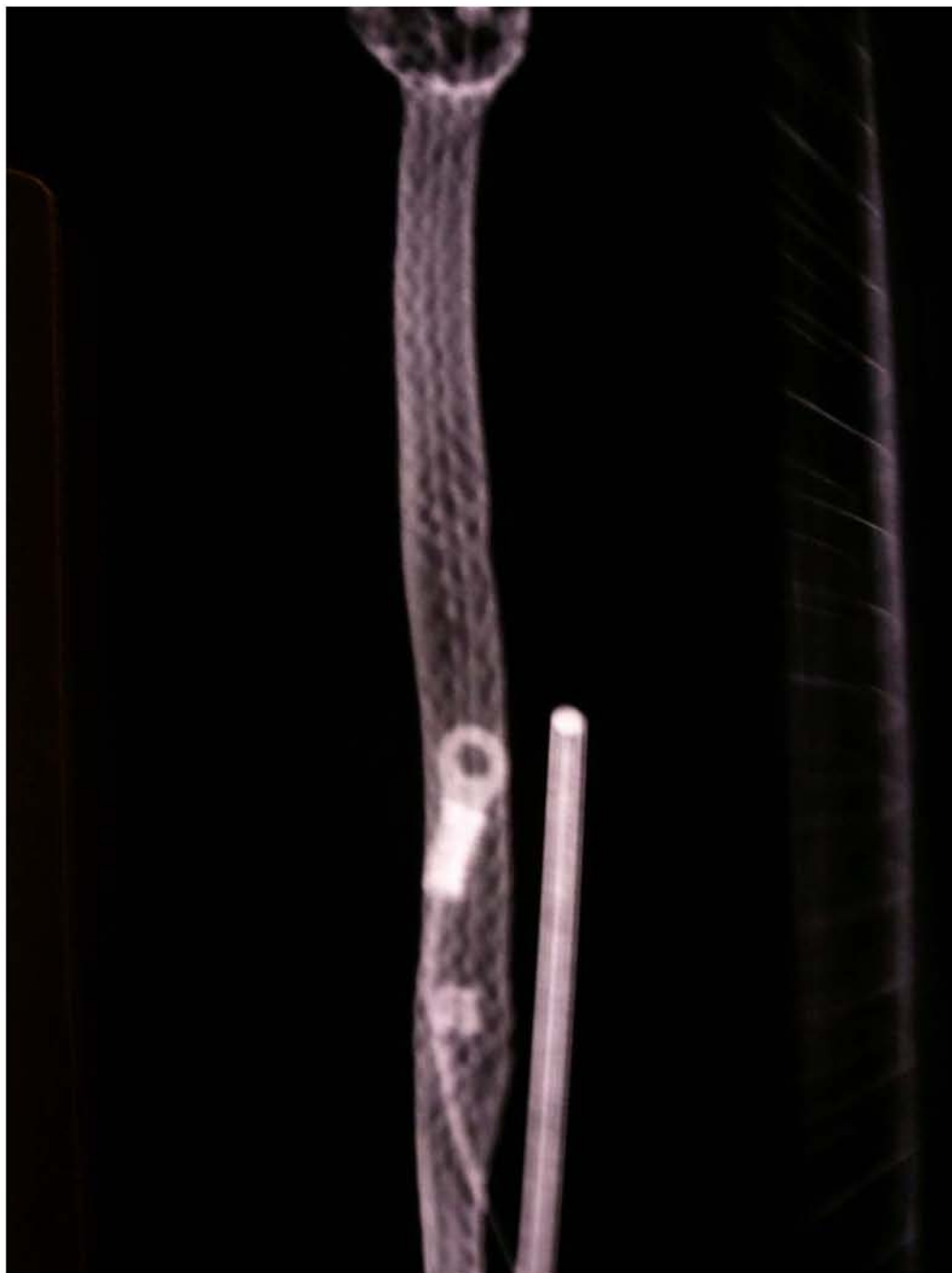
Figure E.95.—Grounding connection for Bulk Fluid Heater 3.
