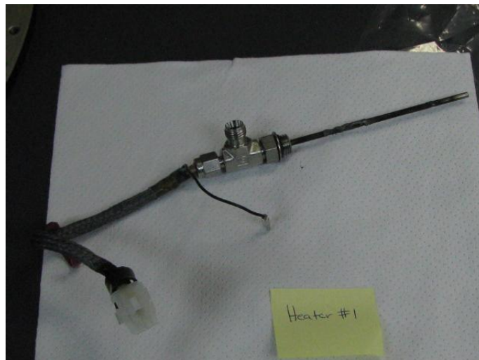
Figure D.14.—Heater 1 extracted with tee from TC, note melted and blackened surface.
