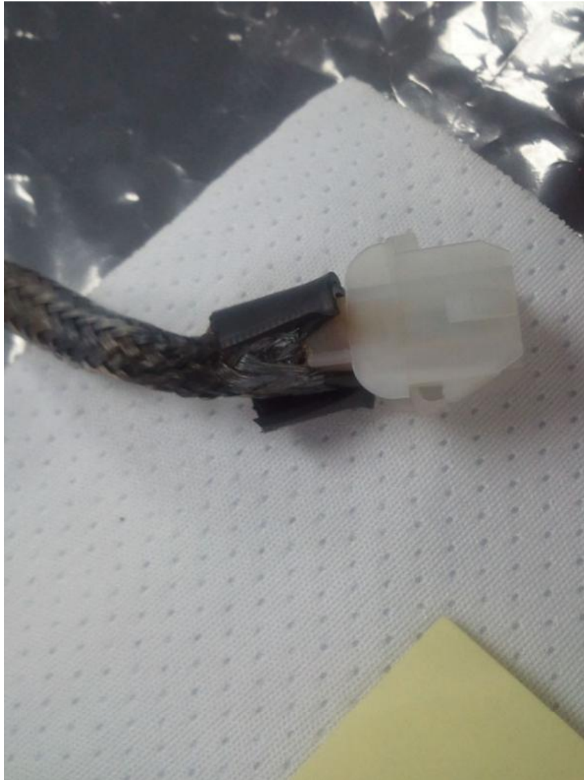
Figure D.48.—Heater 1 Molex connector, note discoloration on wire braid.
