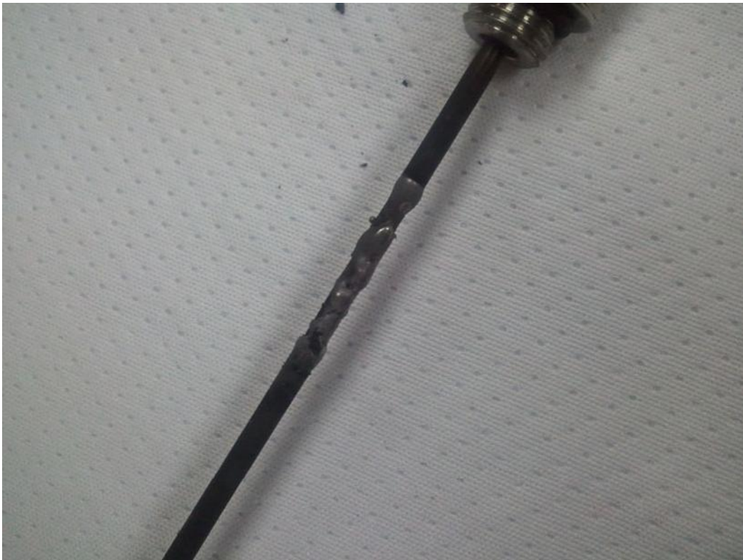
Figure D.40.—Heater 1: Note melted area.
