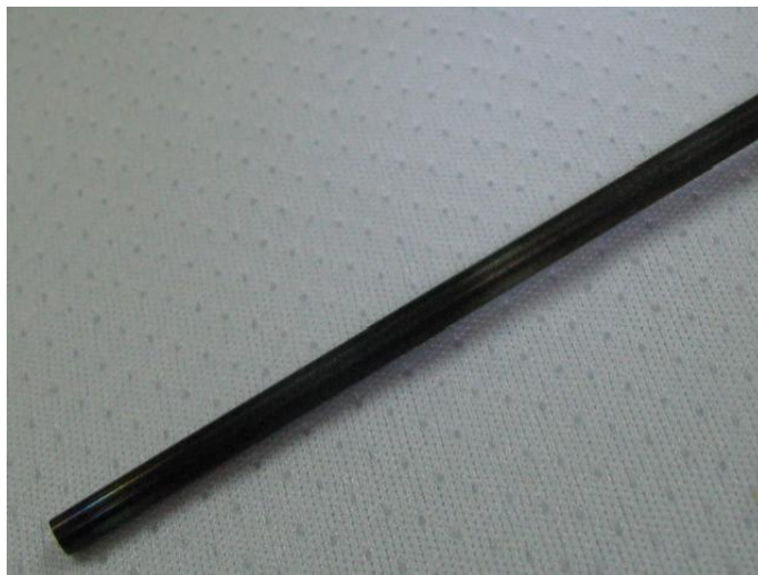
Figure D.65.—Heater 2 fluid immersed portion: Note bluing and blackening.
