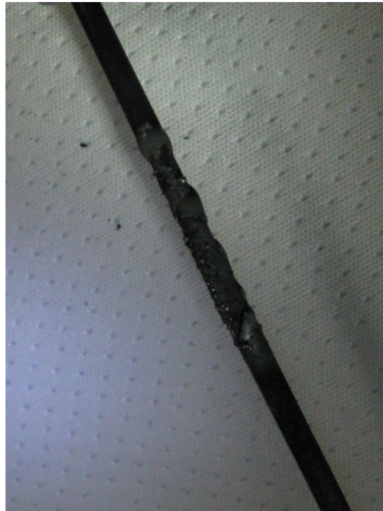
Figure D.16.—Close-up of Heater 1 melted surface.
