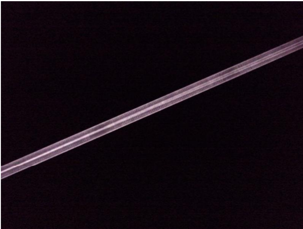
Figure E.61.—Close-up of heating element for Bulk Fluid Heater 2.
