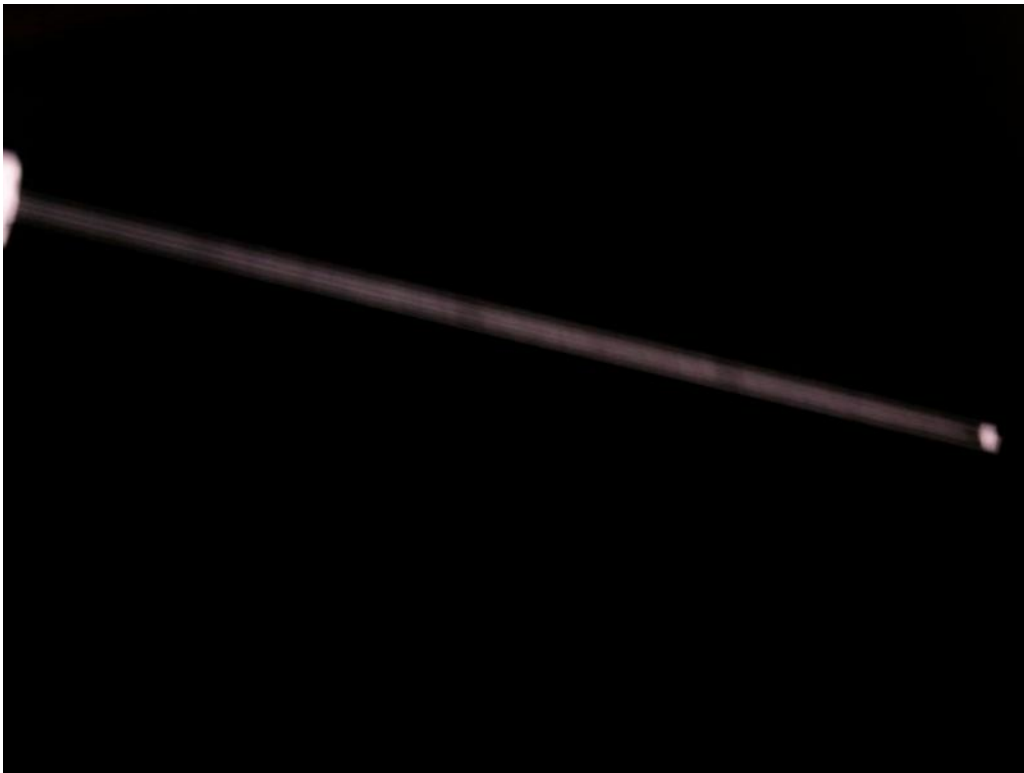
Figure E.73.—Heating element for Bulk Fluid Heater 3. Note irregularities.
