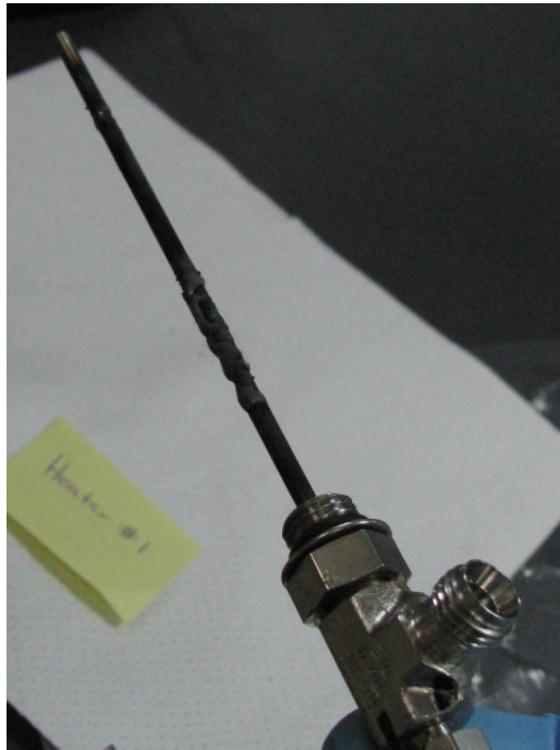
Figure D.31.—Fluid immersed portion of Heater 1: Note two melted areas of Heater 1
