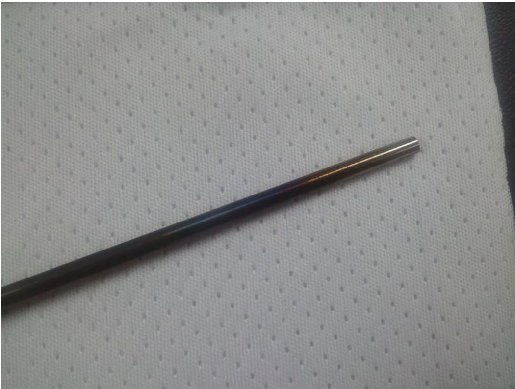
Figure D.92.—Heater 3 fluid immersed portion: Note bluing and blackening.
