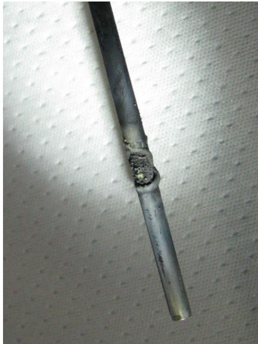
Figure D.17.—Close-up of Heater 1 melted surface near tip of heater.
