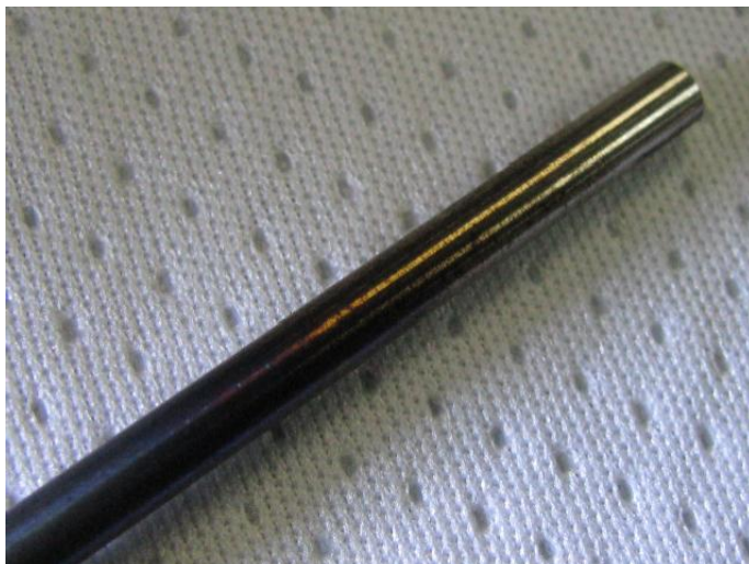
Figure D.88.—Heater 3 fluid immersed portion: Note bluing and blackening.
