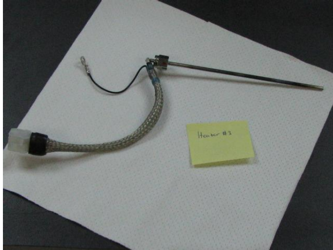
Figure D.83.—Heater 3 assembly: Note bluing and blackening on fluid immersed portion.
