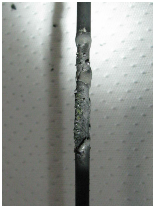
Figure D.18.—Close-up of Heater 1 melted surface.
