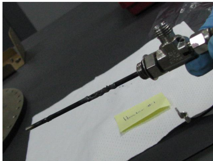
Figure D.32.—Fluid immersed portion of Heater 1: Note two melted areas of Heater 1.
