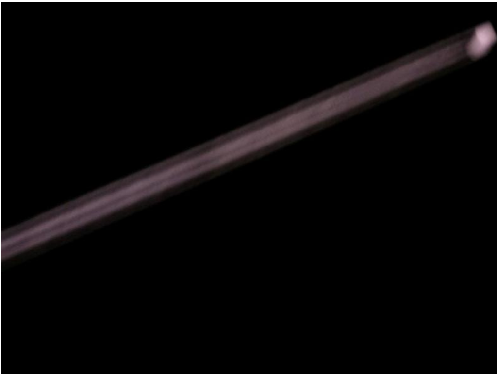
Figure E.51.—Close-up of heating element for Bulk Fluid Heater 2. Note irregularities.
