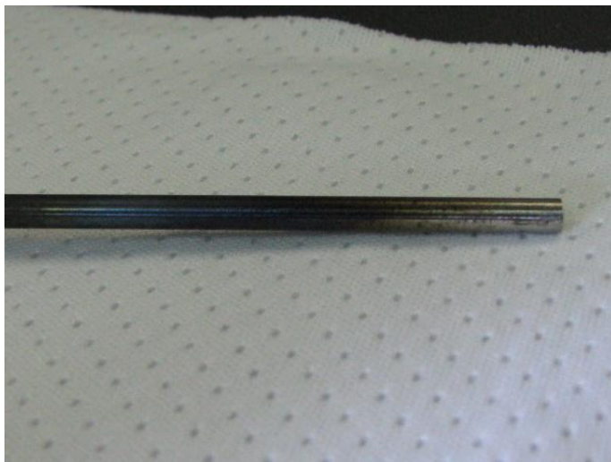
Figure D.89.—Heater 3 fluid immersed portion: Note bluing and blackening.
