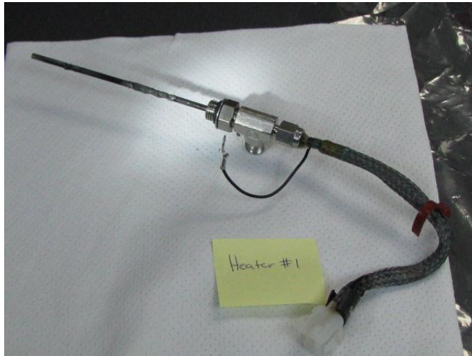
Figure D.15.—Heater 1 extracted with tee from TC, note melted and blackened surface.
