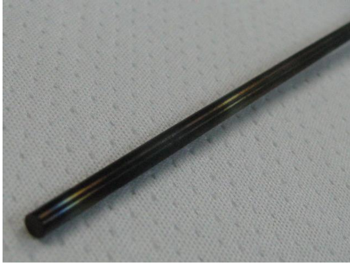
Figure D.66.—Heater 2 fluid immersed portion: Note bluing and blackening.
