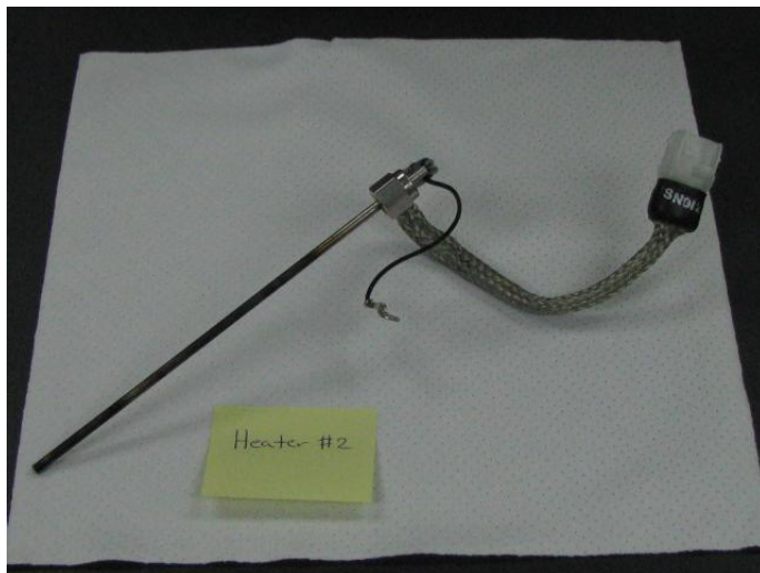
Figure D.69.—Heater 2 assembly: Note bluing and blackening on fluid immersed portion.
