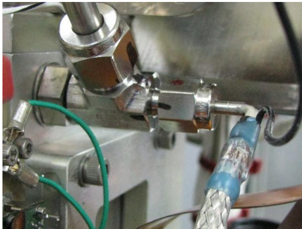
Figure D.76.—Heater 3 connection into TC.
