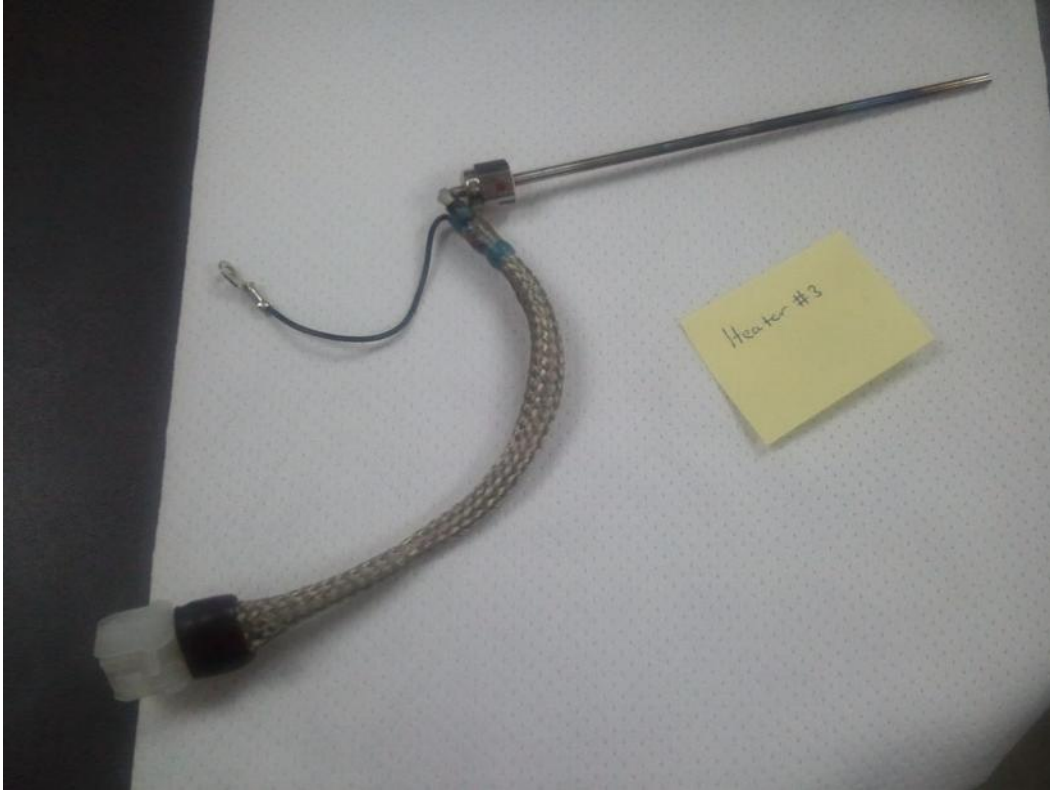
Figure D.91.—Heater 3 assembly: Note bluing and blackening on fluid immersed portion.
