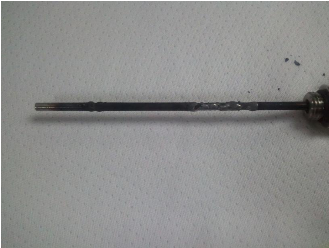
Figure D.38.—Fluid immersed portion of Heater 1: Note two melted areas.
