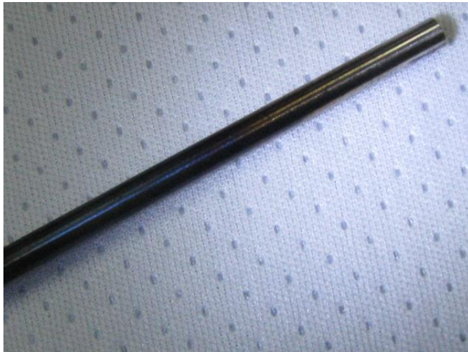
Figure D.87.—Heater 3 fluid immersed portion: Note bluing and blackening.
