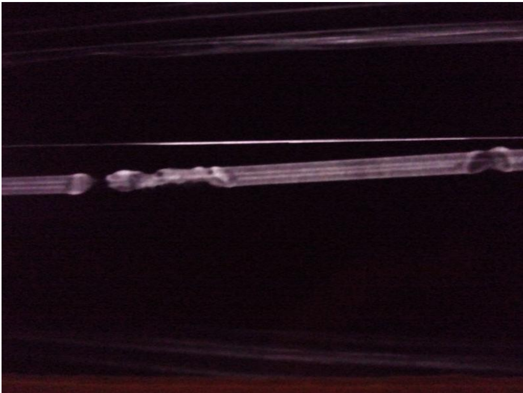
Figure E.7.—Close-up of Bulk Fluid Heater 1 damage along cartridge.
