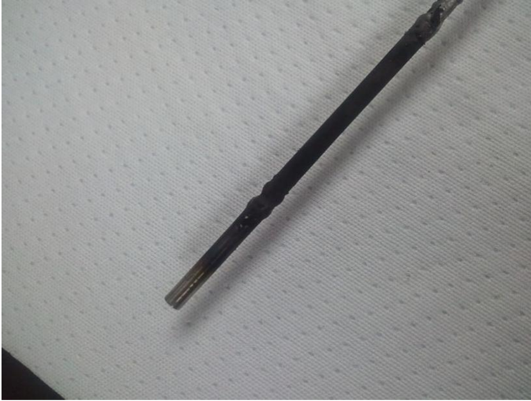
Figure D.41.—Heater 1: Note melted area.
