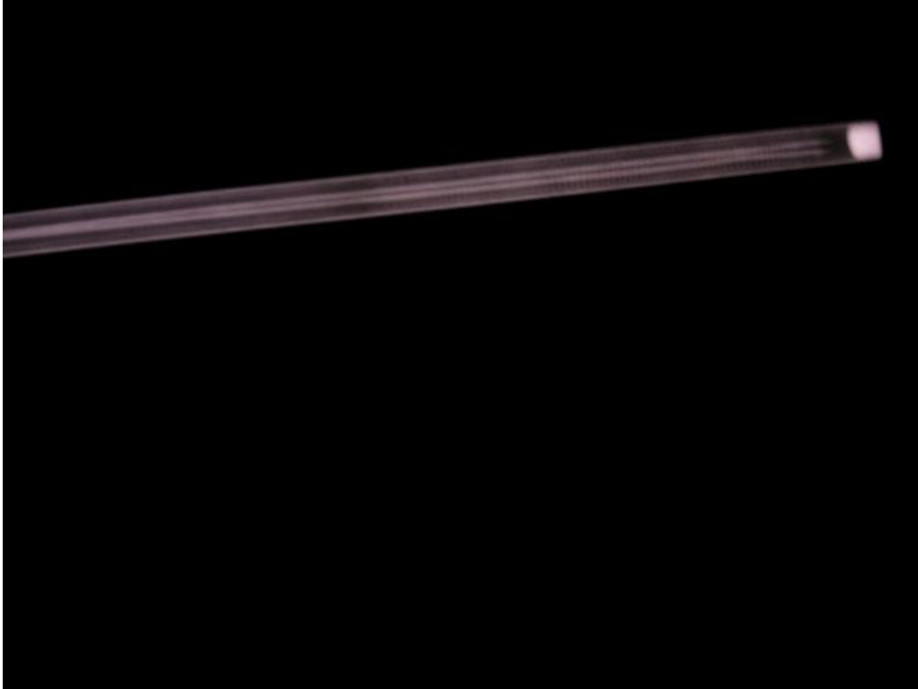
Figure E.54.—Close-up of heating element for Bulk Fluid Heater 2.
