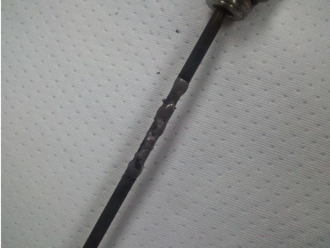
Figure D.39.—Heater 1: Note melted area.
