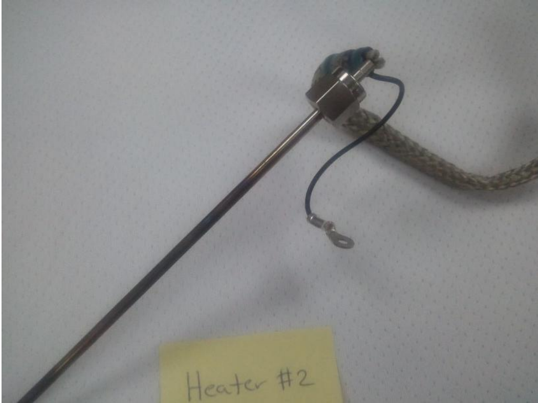
Figure D.71.—Heater 2 assembly: Note bluing and blackening on fluid immersed portion.
