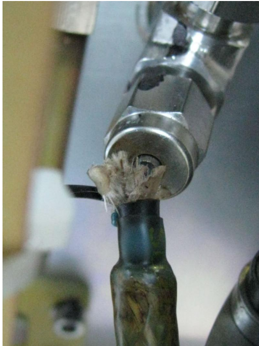
Figure D.7.—Heater 1 feedthrough into TC. Note melted shrink wrap.
