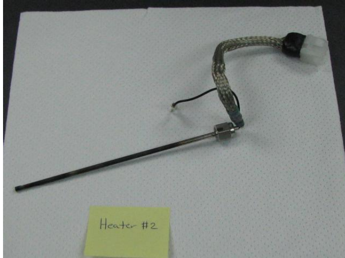
Figure D.63.— Heater 2 assembly: Note discoloration on fluid immersed portion.
