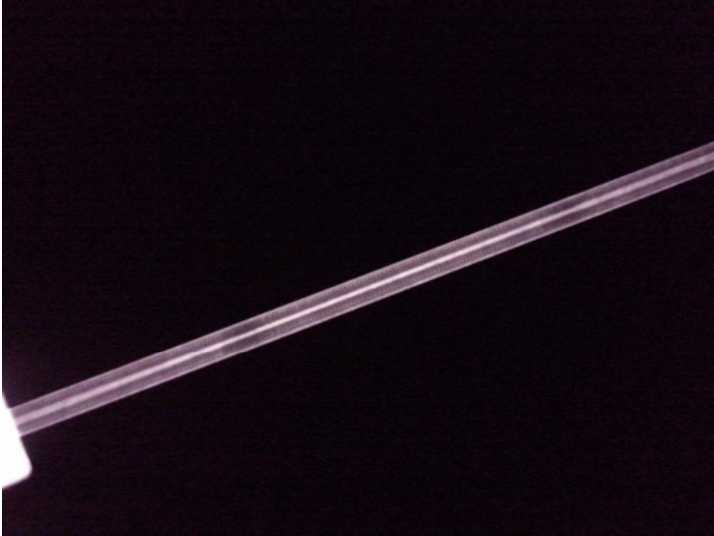
Figure E.62.—Close-up of heating element for Bulk Fluid Heater 2.
