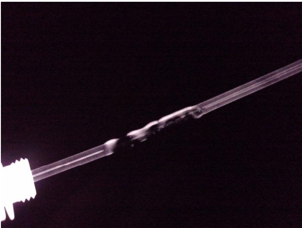
Figure E.39.—Close-up of Bulk Fluid Heater 1 damage along cartridge.
