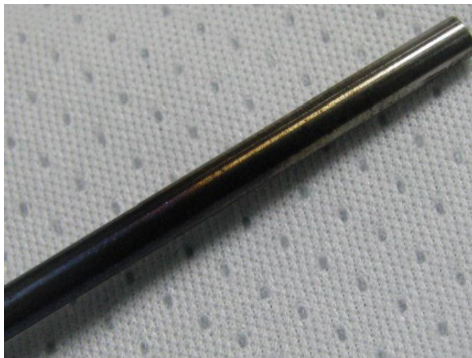
Figure D.85.—Heater 3 fluid immersed portion: Note bluing and blackening.
