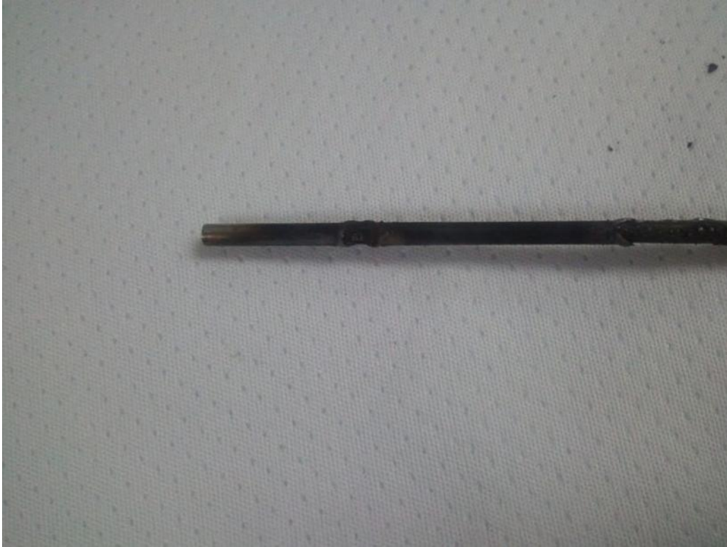
Figure D.45.—Heater 1: Note melted areas.
