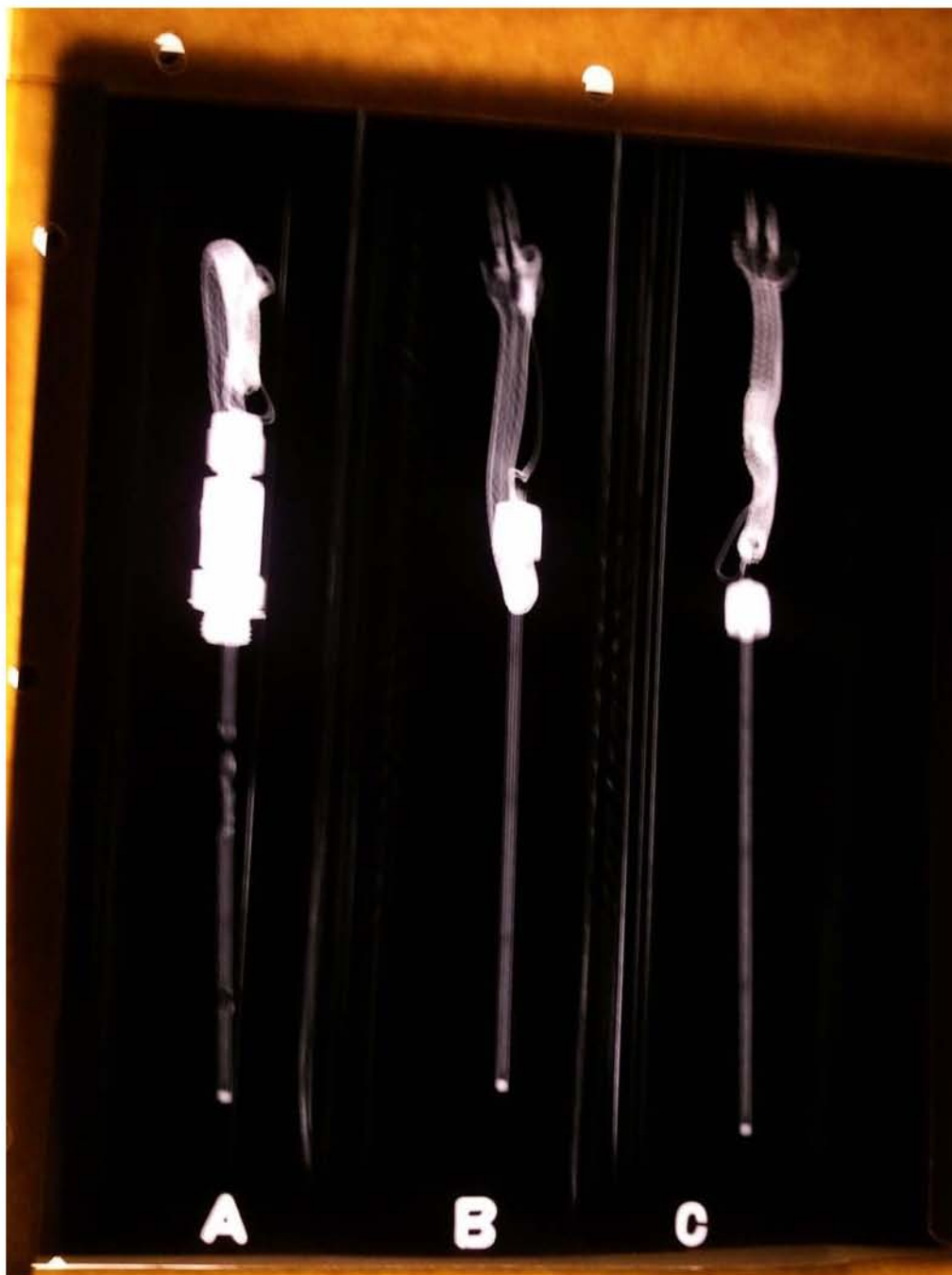
Figure E.3.—Rotated planar view of heater assemblies bulk fluid heaters of 1, 2, and 3, respectively. Note damage in Heater 1.
