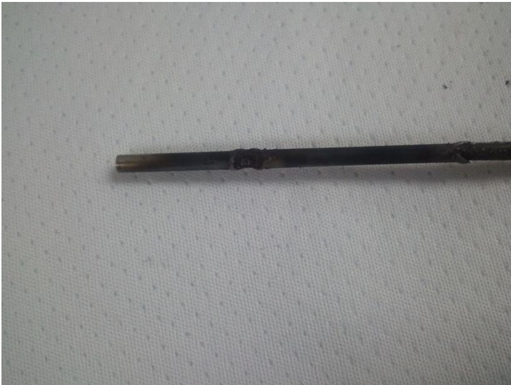
Figure D.46.—Heater 1: Note melted areas.
