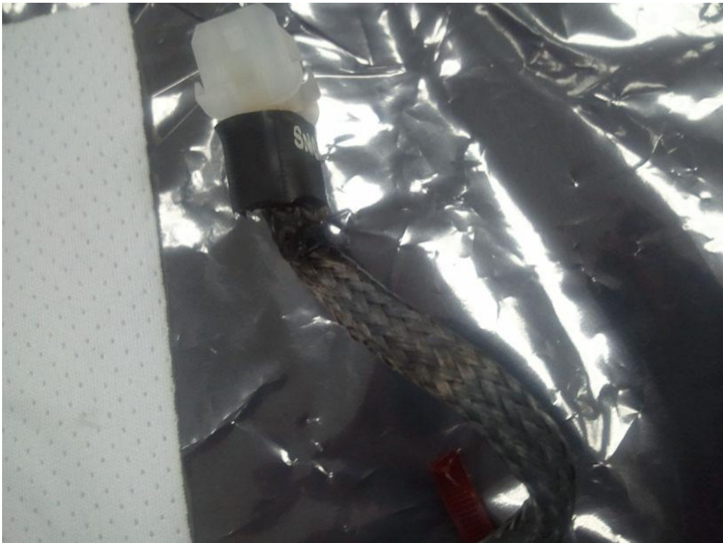
Figure D.54.—Wire harness for Heater 1: Note melted ty-rap and discoloration on wire braid.
