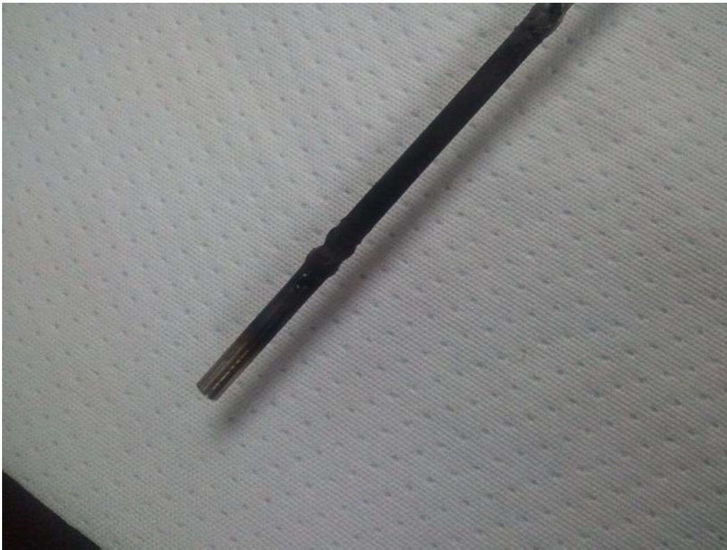
Figure D.42.—Heater 1: Note melted area.
