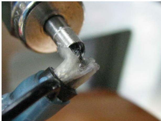
Figure D.74.—Heater 3 connection into TC.
