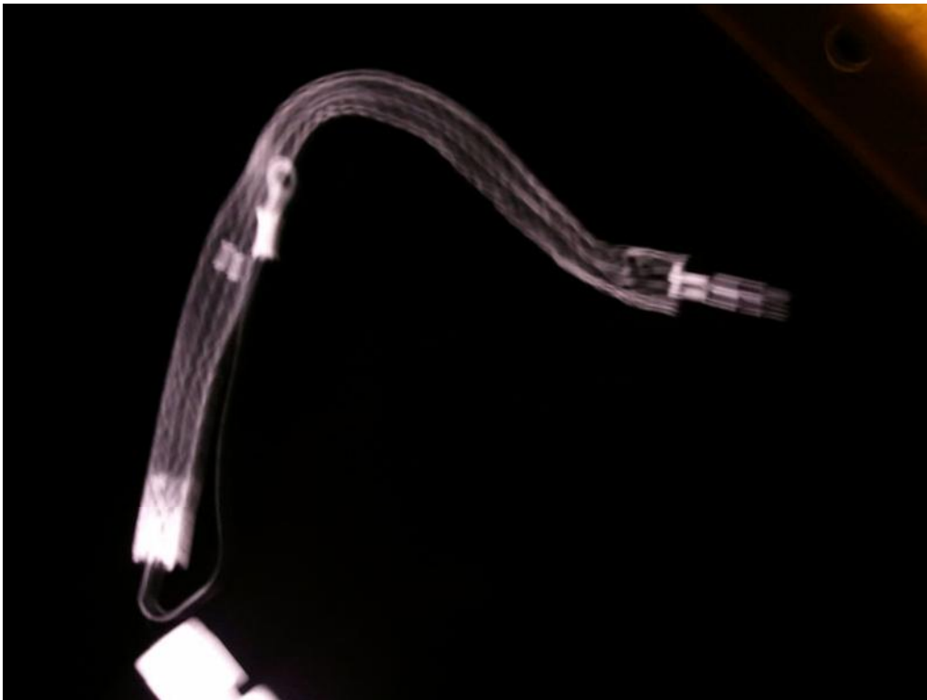
Figure E.31.—Wiring harness for Bulk Fluid Heater 1.
