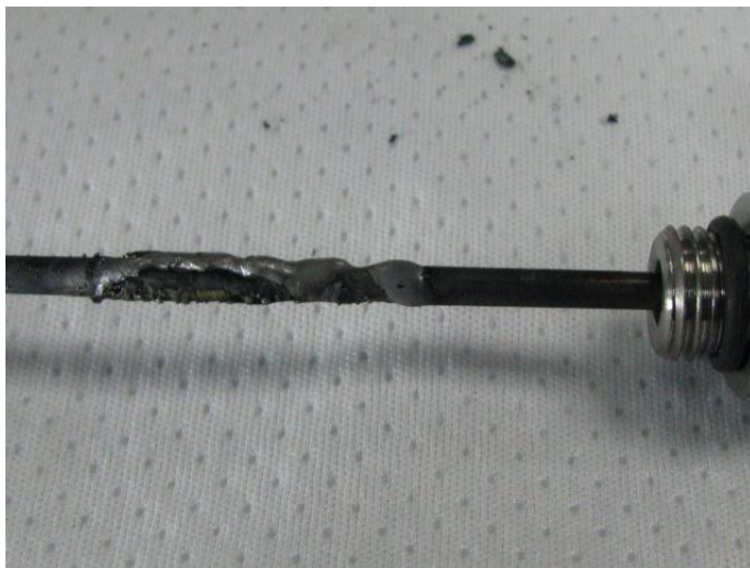
Figure D.24.—Close-up of Heater 1 melted surface.
