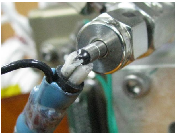
Figure D.77.—Heater 3 connection into TC.
