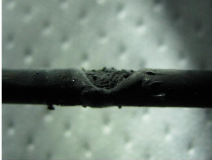
Figure D.28.—Close-up of melted surface near Heater 1 tip.
