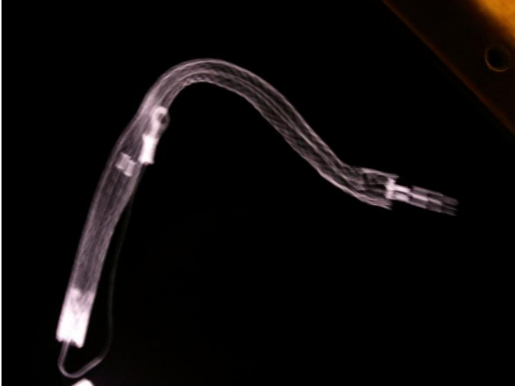
Figure E.30.—Wiring harness for Bulk Fluid Heater 1.
