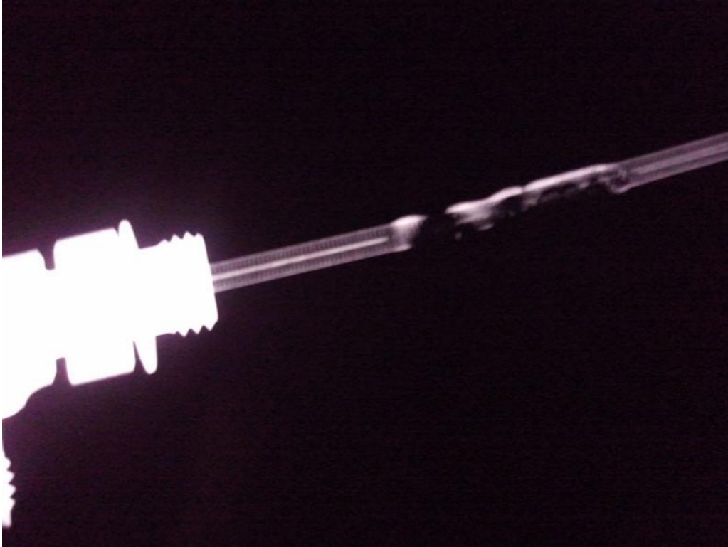
Figure E.40.—Close-up of Bulk Fluid Heater 1 damage along cartridge.
