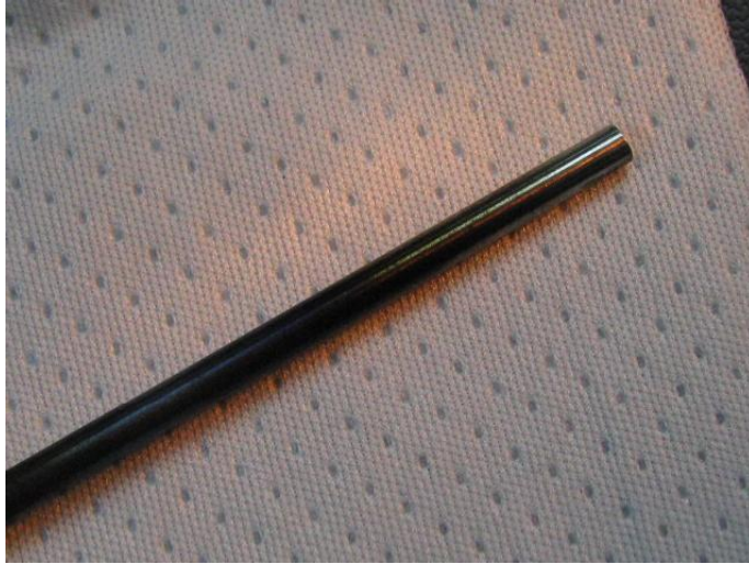
Figure D.86.—Heater 3 fluid immersed portion: Note bluing and blackening.
