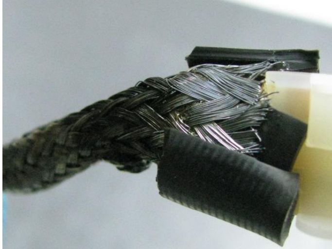
Figure D.5.—Heater 1 Molex connector, strain relief sliced open, note discoloration on wire braid.
