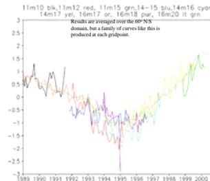
Curve segments which approximate AM-PM drift rates are independent of each other. Because the PM sensors share a similar diurnal drift rate, where the segments overlap in time they should have the same offset value. We thus (arbitrarily) adjust the curves segments using n11 as the reference.
