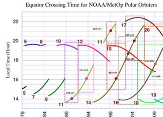
Equatorial crossing times for NOAA operational polar orbiting satellites. Dashed lines indicate temporal segments of overlap where the PM satellites (n11, n14, n16) are drifting rapidly compared to other satellites. Dots indicate the mid-points of these periods.
