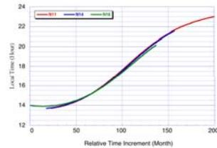
Similarity in relative drift rates of equatorial crossing times enable parameterization of correction
