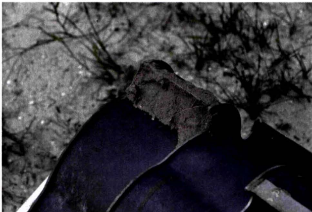
Figure 13 – Scoop clogged with damp sand.
