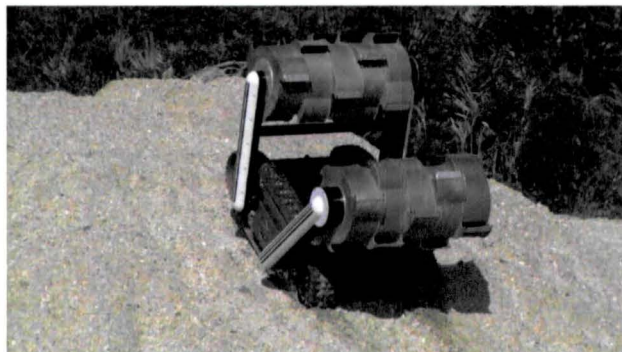
Figure 6 – Driving up a 20 degree slope of loose crawler-way fines.
