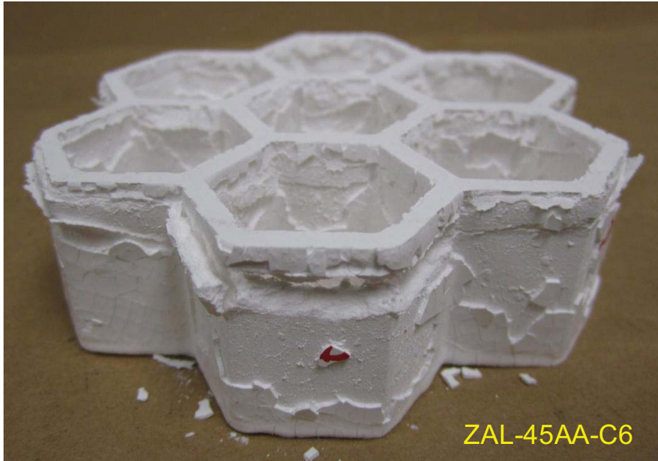
Figure 11. ZAL-45AA honeycomb core flatwise compression specimen after test.
