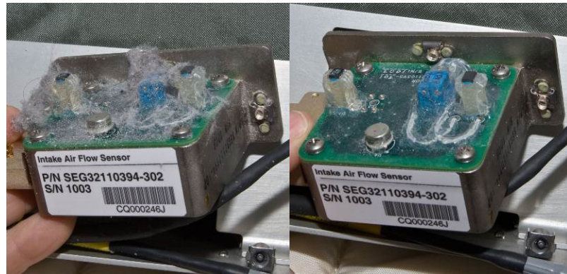
Figure 2. Starboard CQ intake air flow sensor (pre and post cleaning).
