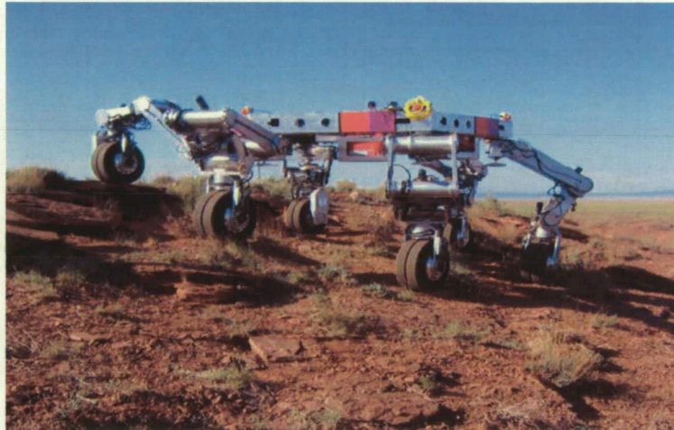
Figure 8. A one third scale ATHLETE undergoing tests in a desert analog lunar environment. (Ref 3)
