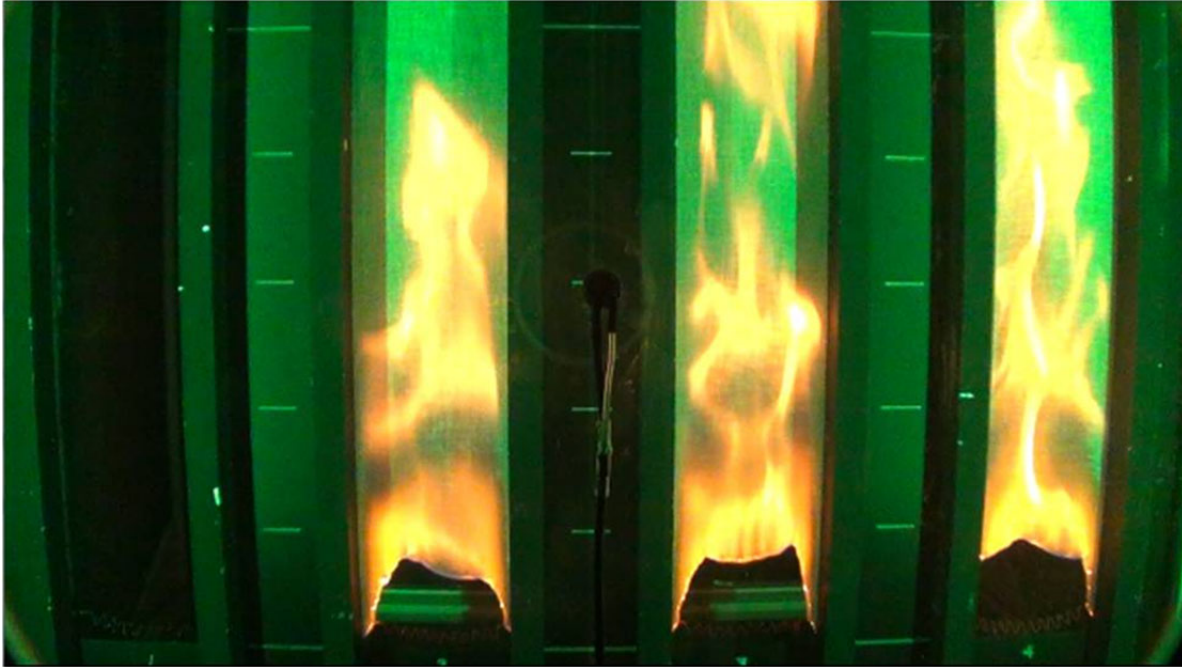
Figure 49.—Three sample cheesecloth, bottom simultaneous ignition, with quench bars.
