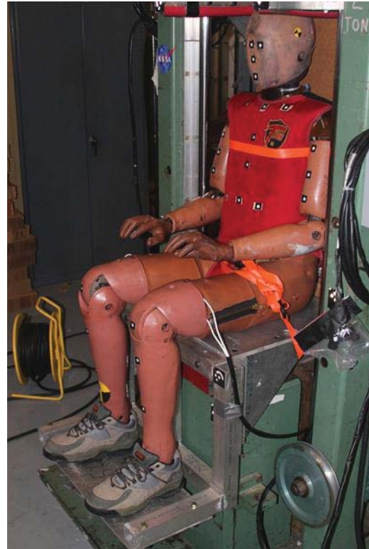
Figure 21- THOR test setup with footrest
