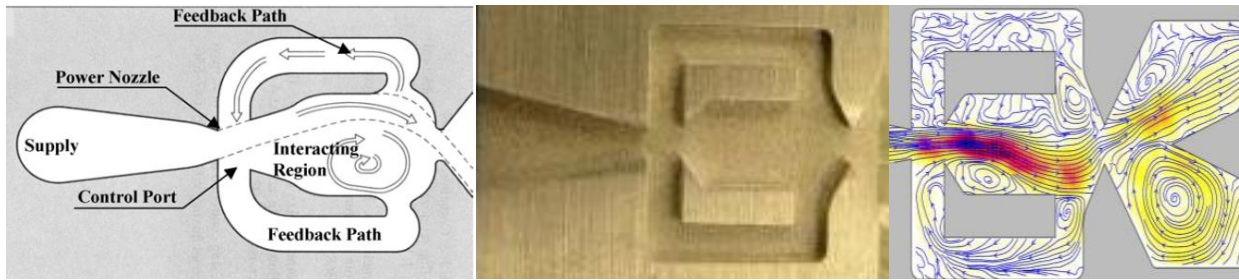
Figure 7 Typical sweeping jet actuators and the interior flow in them [23].
