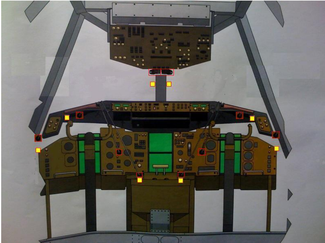
Figure 45. Location of Oculometers and IR Flashers in IFD Simulator
