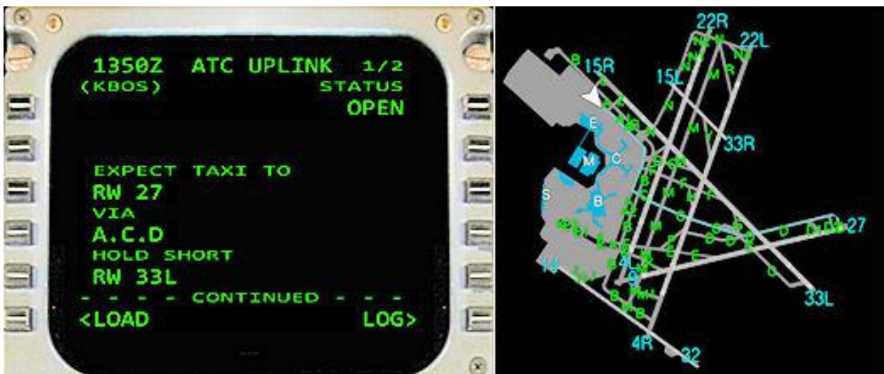
Figure 9. Open Expected D-TAXI message on CDU (left) and display on ND (right)
