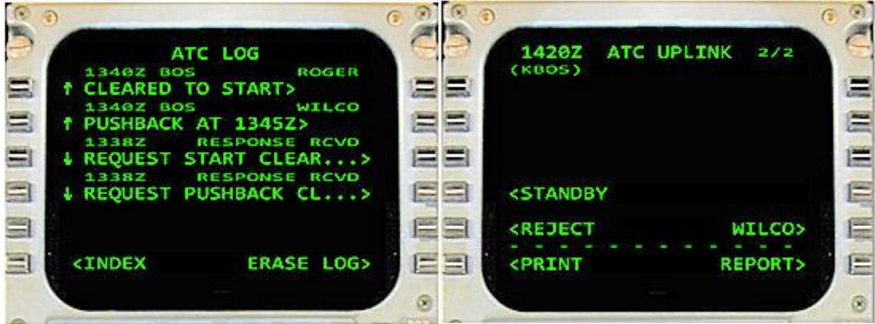
Figure 8. ATC Log (left) and Downlink Response (right) pages
