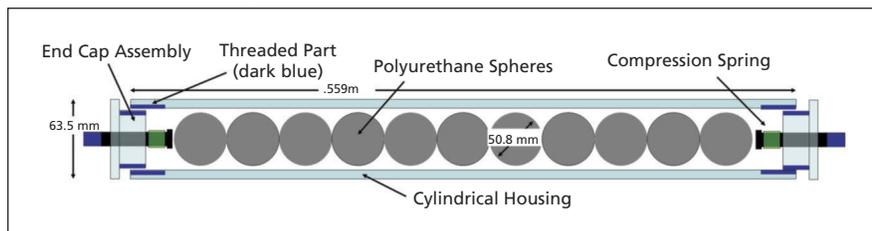
Figure 1. Initial schematic for the **Vibration Suppressor**. Pistons at each end of the cylinder make contact with the granular chain of spheres. Static compression of the granular chain is achieved through the use of soft springs located between the pistons and end caps, which screw onto the container.
