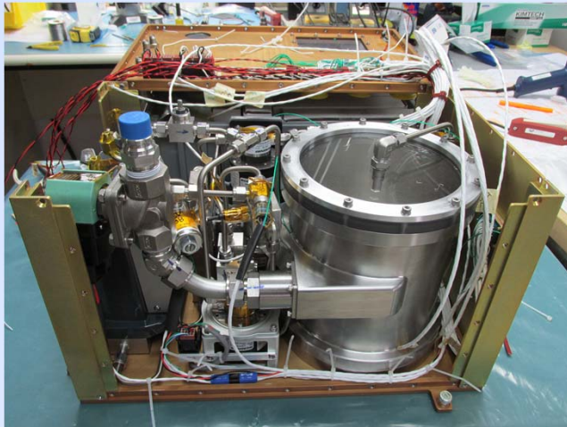
Pumped Separator for PBRE
