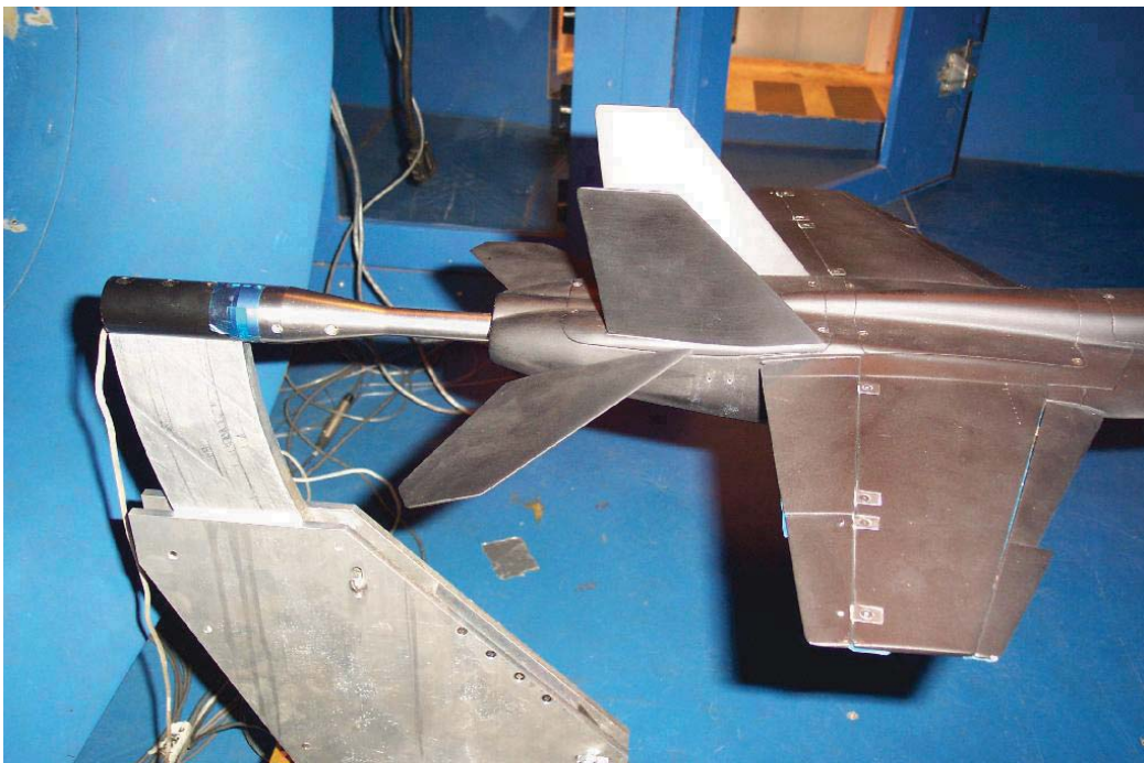
(b) close-up view of the right horizontal stabilizer at +20-degrees incidence
