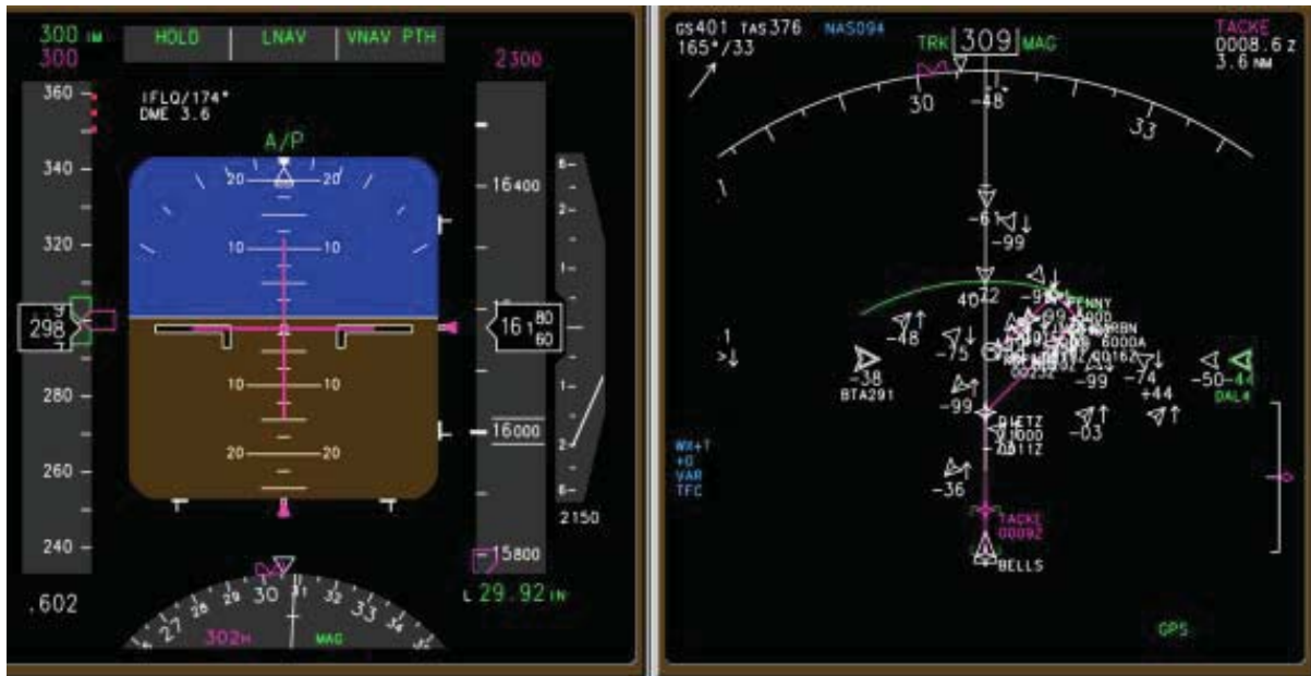
Figure 9. PFD and ND with FIM information (single-pilot simulator).
