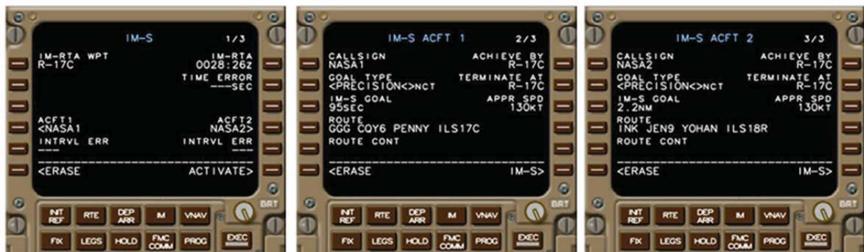
Figure 6. CPDLC FIM clearance on MCDU pages (two-pilot simulator).
