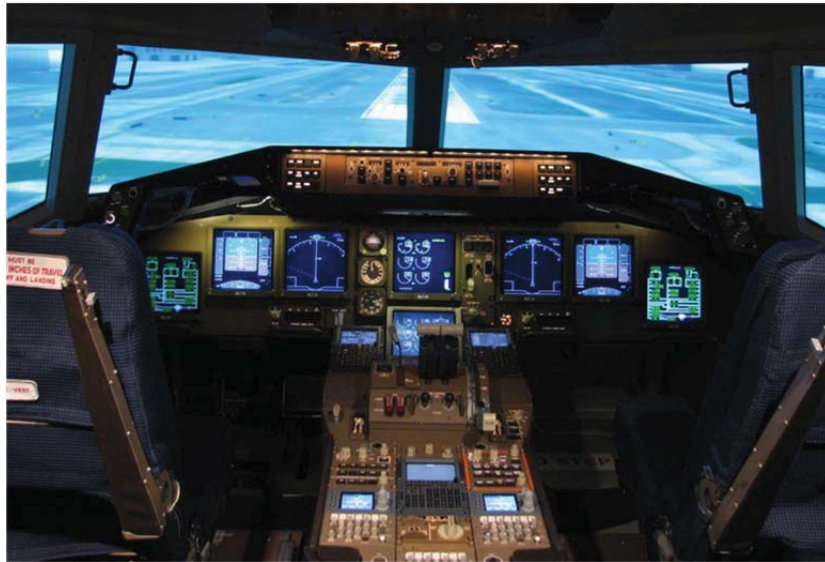
Figure 11. Development and Test Simulator (DTS).
