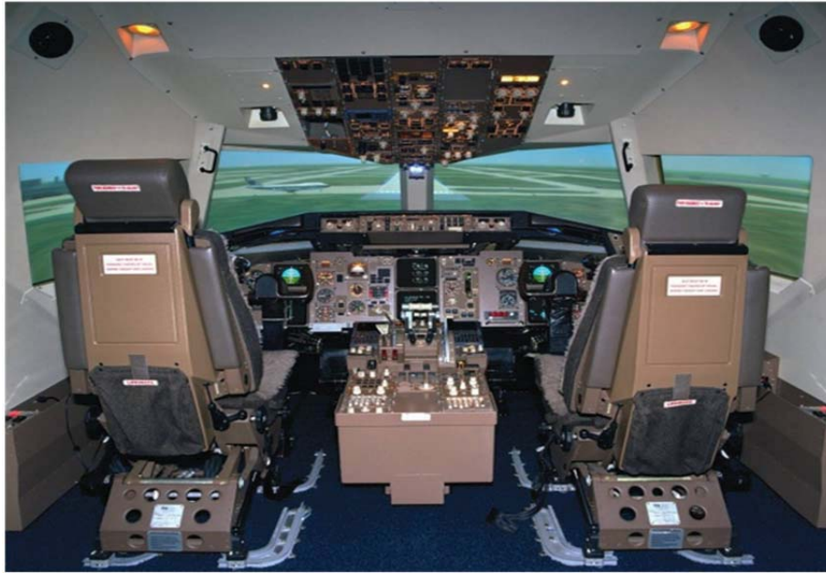
Figure 12. Integration Flight Deck (IFD) simulator.
