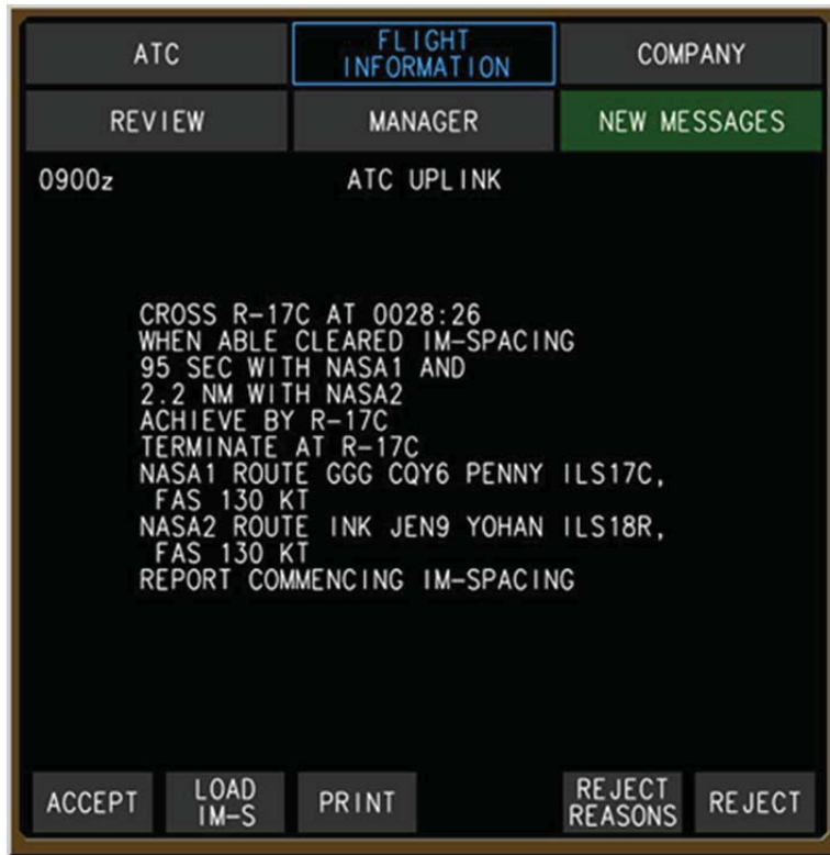
Figure 5. CPDLC FIM clearance on an EICAS page (single-pilot simulator).
