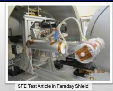
Thrust magnitude increased over multiple test devices from 16 to 170mN
