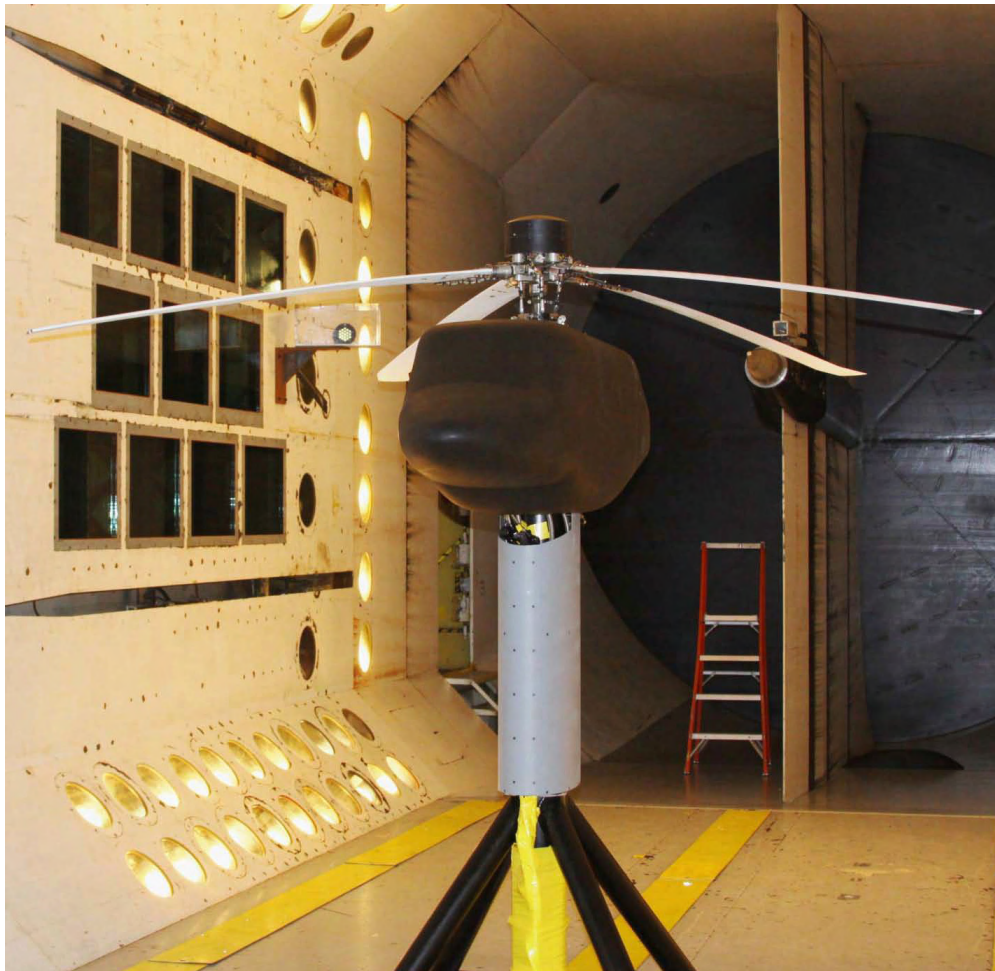
Figure 1. ARES/ATR model in the Transonic Dynamics Tunnel.
