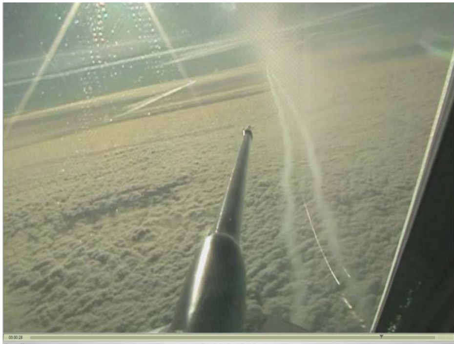
Figure 7.1-14. DLR Video Screen Grab showing Diffuse Exhaust Contrail above A-340 Wake Vortices
