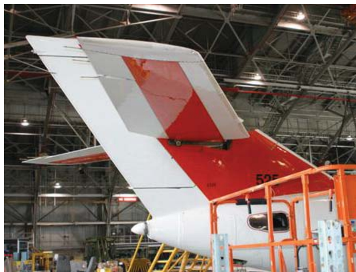
Figure 6.1-9. Falcon 20 Cruciform Tail, Left Side with Access Panels Removed
