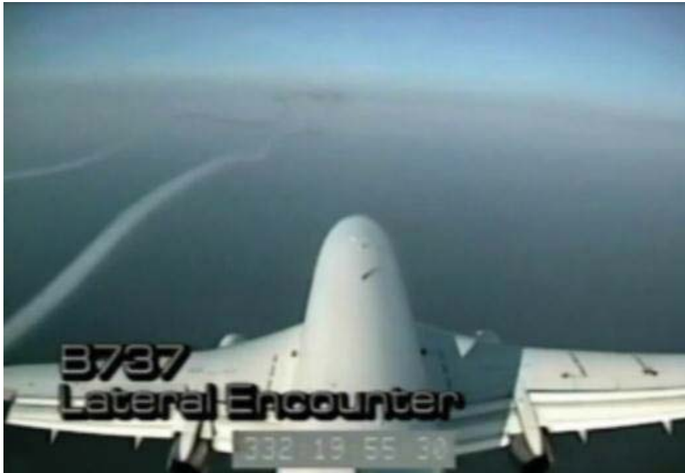
Figure 7.1-11. B-737 Approaching C-130 Vortex Pair in Far Field
