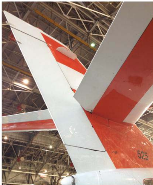
Figure 6.1-8. Falcon 20 Cruciform Tail, Left Side with Access Panels Installed
