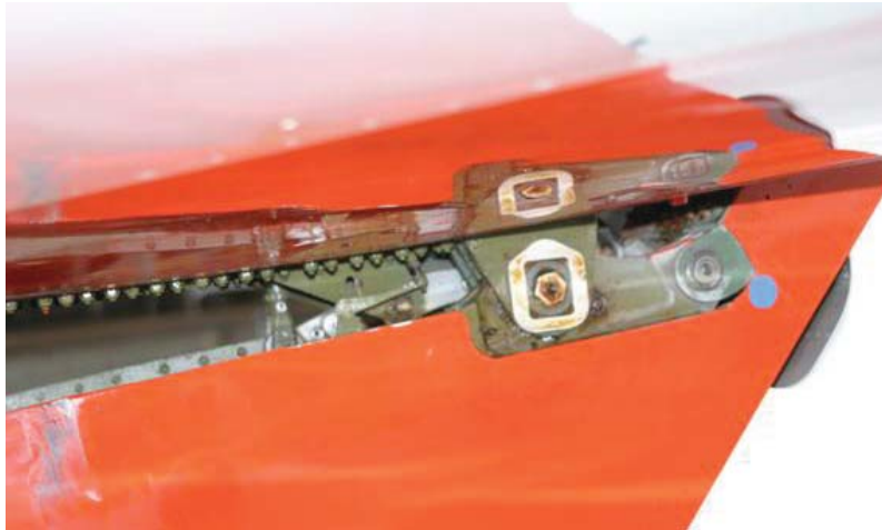
Figure 6.1-10. Falcon 20, Right-side Horizontal Tail Aft Connection
