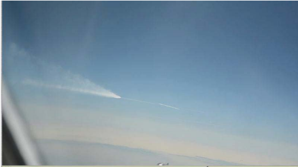
Figure 7.1-12. DLR Video Screen Grab showing Far-Field Separation: Diffuse Exhaust Contrail above Wake Vortices
