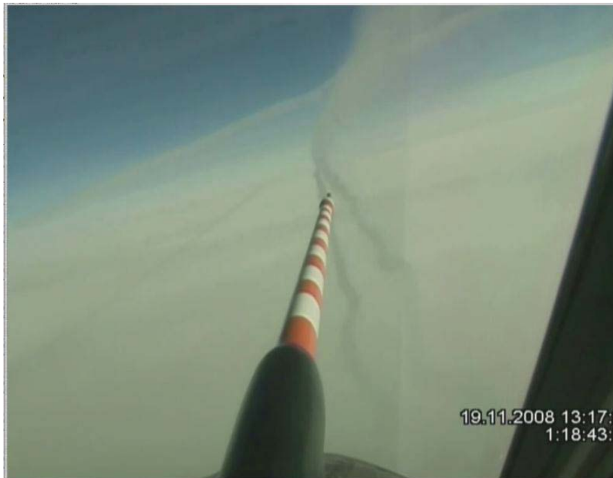
Figure 7.1-13. DLR Video Screen Grab showing Diffuse Exhaust Contrail above A-380 Wake Vortices
