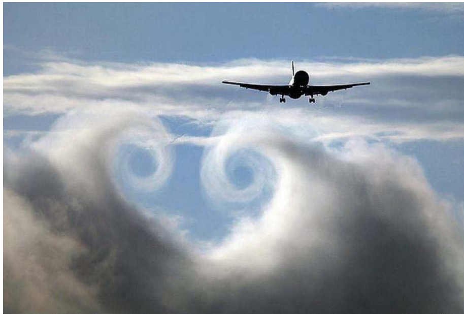
Figure 7.1-2. Photograph of Merging Exhaust and Vortex Pair from Transport Airplane in Landing Configuration at Unknown Speed and Altitude
