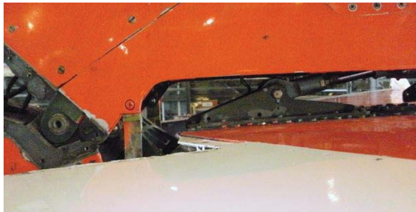
Figure 6.1-11. Falcon 20, Right-side Horizontal Tail Forward Connection
