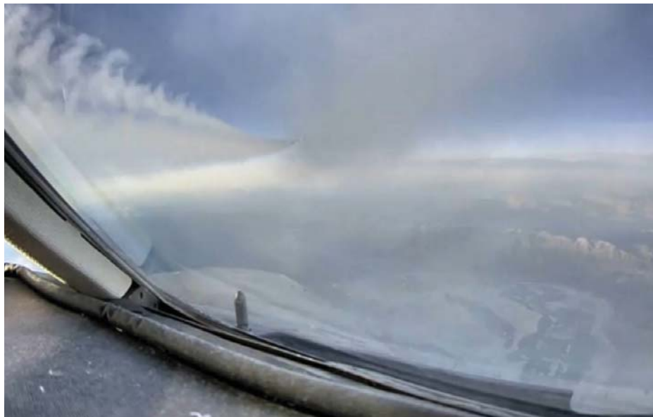
Figure J-4. Pilot Proficiency Practice April 2013: Immersed in Right Inboard Exhaust Contrail; Left Wingtip Vortex is Made Visible by the Rolled Up Left Outboard Exhaust Contrail; Located to the Left and “Centerline At Least One Core Diameter (~6 feet) Above” the Centerline of the Left Inboard Exhaust Contrail; Right Wingtip Vortex Obscured
