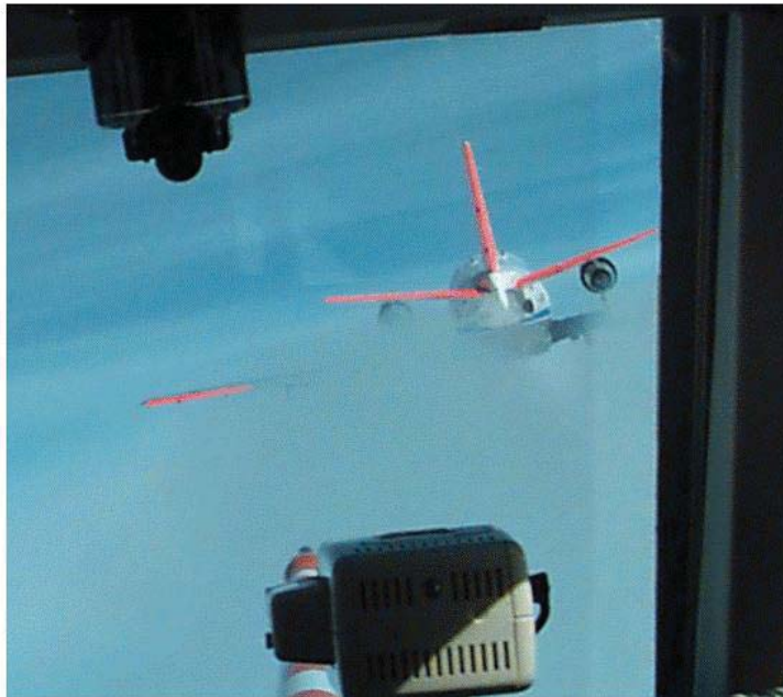
DLR Falcon Sampling NF behind a VFW-Fokker 614 (WS 70.5 ft)
