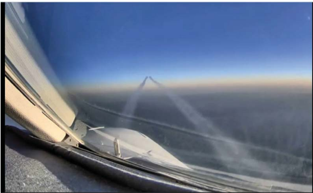
Figure J-7. Pilot Proficiency Practice April 2013: Approximately 300 ft Above the Vortices in Far Field; Both Cores are Made Visible by Rolled up Exhaust Contrails
