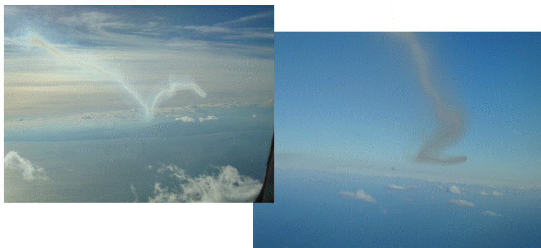
Illustrations of Chaotic Nature of Single FF WVC Made Visible by Injecting Oil into Outboard Engine Exhaust Plume
