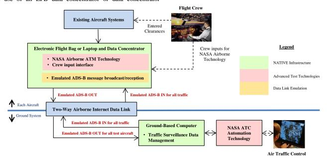
Figure 1: A potential NATIVE test configuration for a concept that uses ADS-B for airborne surveillance.
