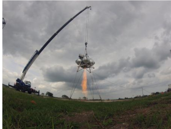
Figure 5 – Morpheus in standard Hot-fire Test Configuration
