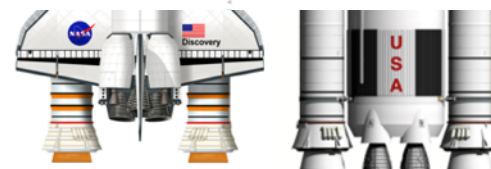
SLS Main Engine proximity to Booster Thermal Curtain results in increased loads (over SSME loads)
