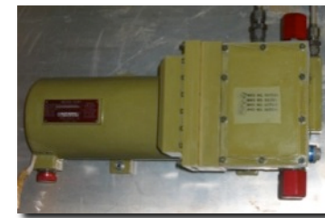
Shuttle Hydraulic Recirculation Pump
