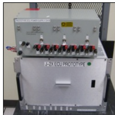
RS-25 ECU Basic design supports RS-25 and J-2X
