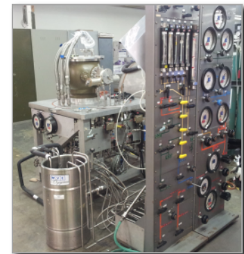
Prevalve Bench Testing on Common Cryo Test Stand
