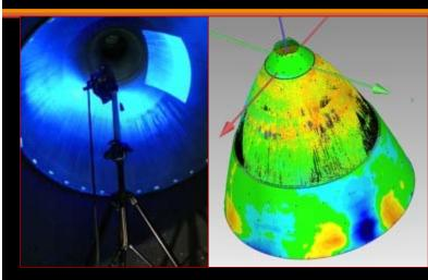
Replaced difficult measurements with scanning to ( help **reduce performance uncertainty** (throat and exit areas) Training and Implementing as a new technique for Rocketdyne Personnel
