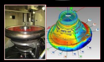
Structured light used to generate machining code and match machine at PWR
