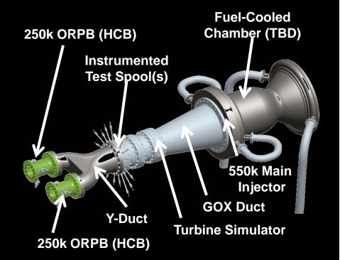
Testing planned for FY16 at NASA Stennis test stand E-1
