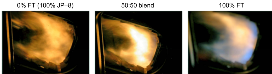
Figure 7.—Digital camera photographs showing flame changes with changes in fuel blend at fuel:air ratio F/A = 0.020 . JP-8 fuel is visibly more luminous.
