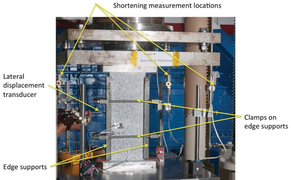
Fig. 4. Specimen in test machine and displacement measurement locations.
