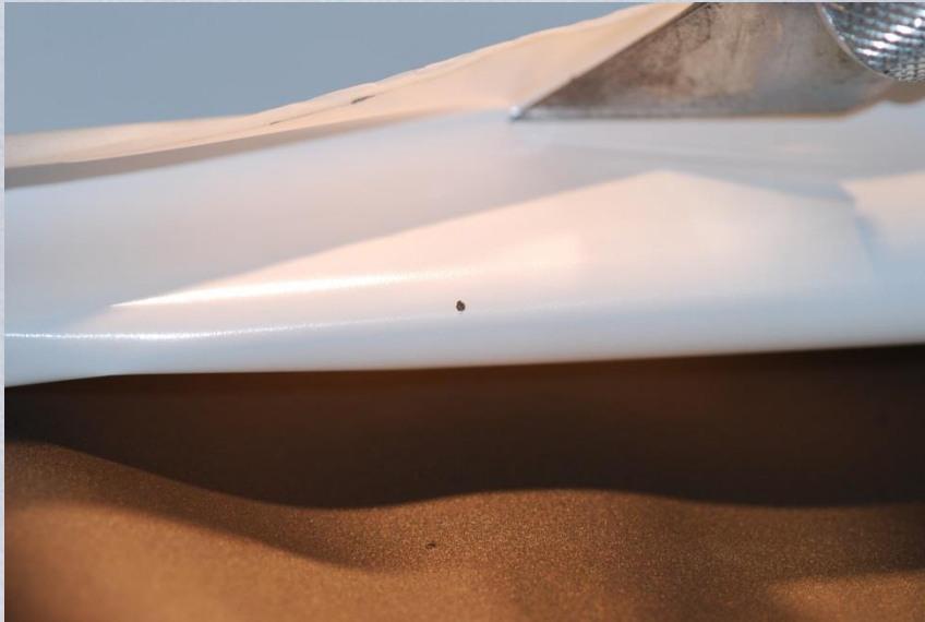
Active material bump on anode coating
