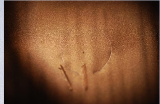
Active material deposit on cathode side of separator
