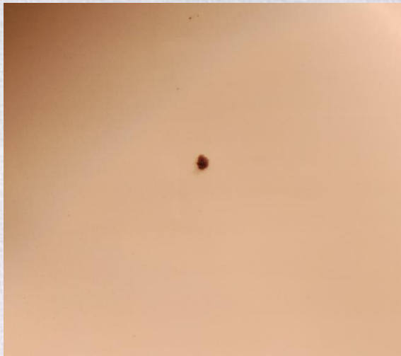
Active material bump on anode coating
