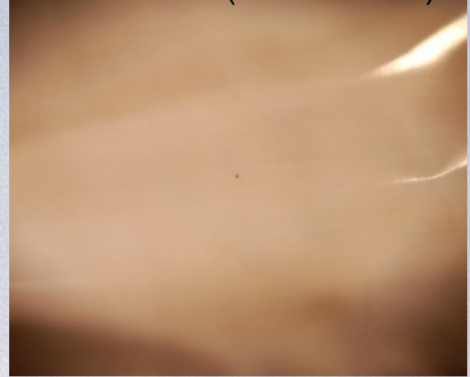
Active material deposit on cathode side of separator
