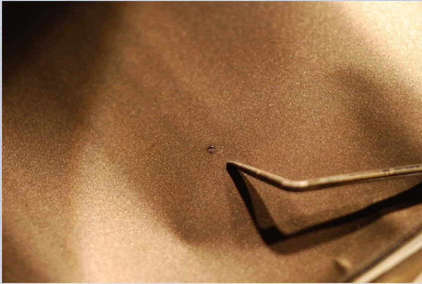
Active material bump on anode coating
