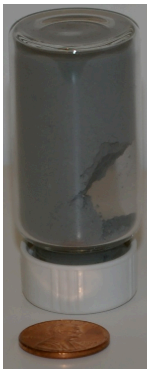
Figure 5. Glass used in the Chenobi simulant after milling with the Zybek mill. The material is highly resistant to slump, presumably due to a very high particle angularity.
