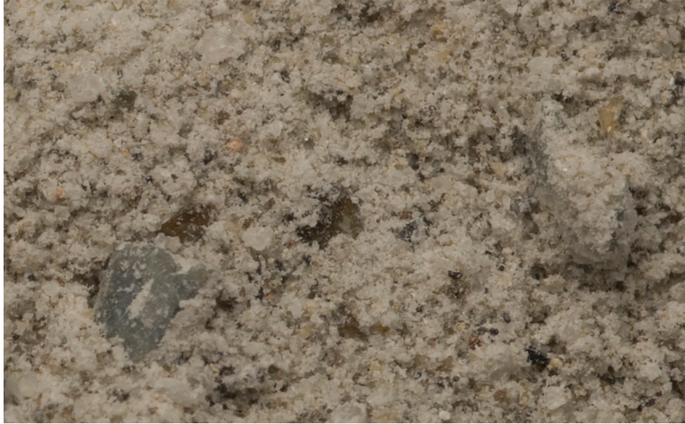
Figure 4. Photomicrograph of NU-LHT-2M in plain light. The large particle in the lower left is approximately 1 mm long.
