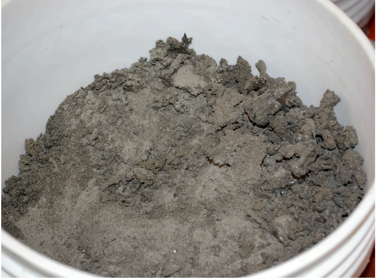
Figure 11. Five-gallon bucket of pseudo-agglutinate produced by Zybek. Visually the material is a mixture of mill sand and vesicular glass in varying proportions.
