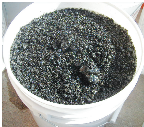
Figure 9. Glass produced from melting of mill sand. This product is referred to as 'high quality glass.'
