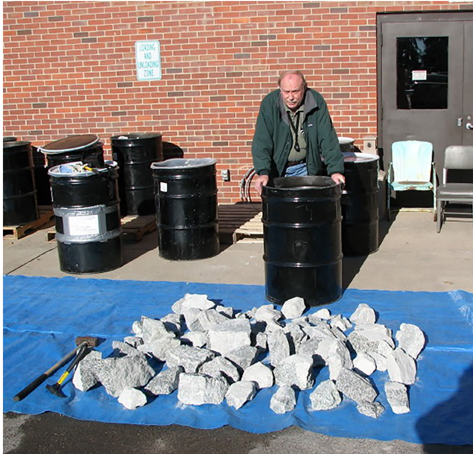
Figure 19. Doug Stoesser with typical material received at the USGS facility in Denver from the Stillwater mine. Shipments used both 55-gal drums, as in this case, and 1 m 3 containers made at the mine site from containers used to ship milling chemicals. These rocks are dominantly norite and anorthosite and have not yet been washed.
