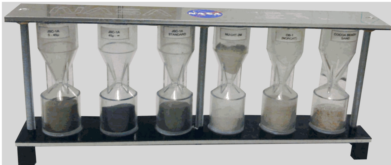
Figure 2. Comparison of the flow characteristics of simulants. From left: JSC-1A <45 µm, JSC-1A >45 µm, JSC-1A, NU-LHT-2M, OB-1, and Coco Beach Sand. NU-LHT-2M did not flow through the orifice under the test conditions. Also note the difference in adhesion as can be seen in the amount of discoloration in the upper chamber. Image provided by Robert P. Mueller of KSC.
