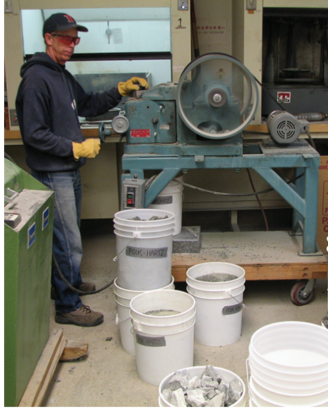
Figure 20. Jaw crusher: (a) Steve Wilson operating the 6-in jaw crusher. Material in the foreground bucket has yet to be run through the crusher. Material in the two buckets on the floor have been through the crusher, and (b) overhead oblique view of jaw crusher. The arrow marks the moving jaw, which is inside the in-feed opening of the machine.
