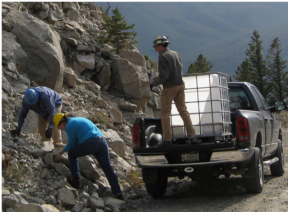
Figure 16. Selecting and collecting rock: (a) From the waste pile of the mine. In the middle ground, behind the bin, one of the mine personnel is washing rock to make identification of acceptable material easier (note the use of personal safety equipment), and (b) from a road cut above the mine where norite is being collected. The small rocks visible in this photo are not optimally sized but are of good mineralogical quality.
