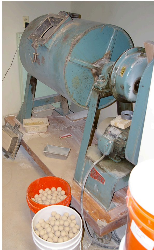
Figure 21. Ball mill with two 5-gal buckets of aluminum oxide ceramic grinding media in the foreground. Rock to be ground and the grinding media are poured into the port visible on the top quadrant of the rotating drum.
