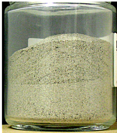
Figure 3. Segregation and stratification in NU-LHT-1M after handling.
