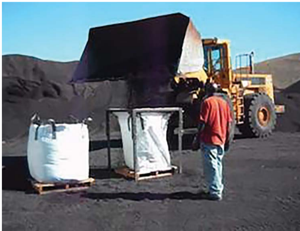
Figure 2. Loading of super sacks at the Miller Mining facility northeast of Flagstaff, AZ (image from Zybek Advanced Products; used with permission).
