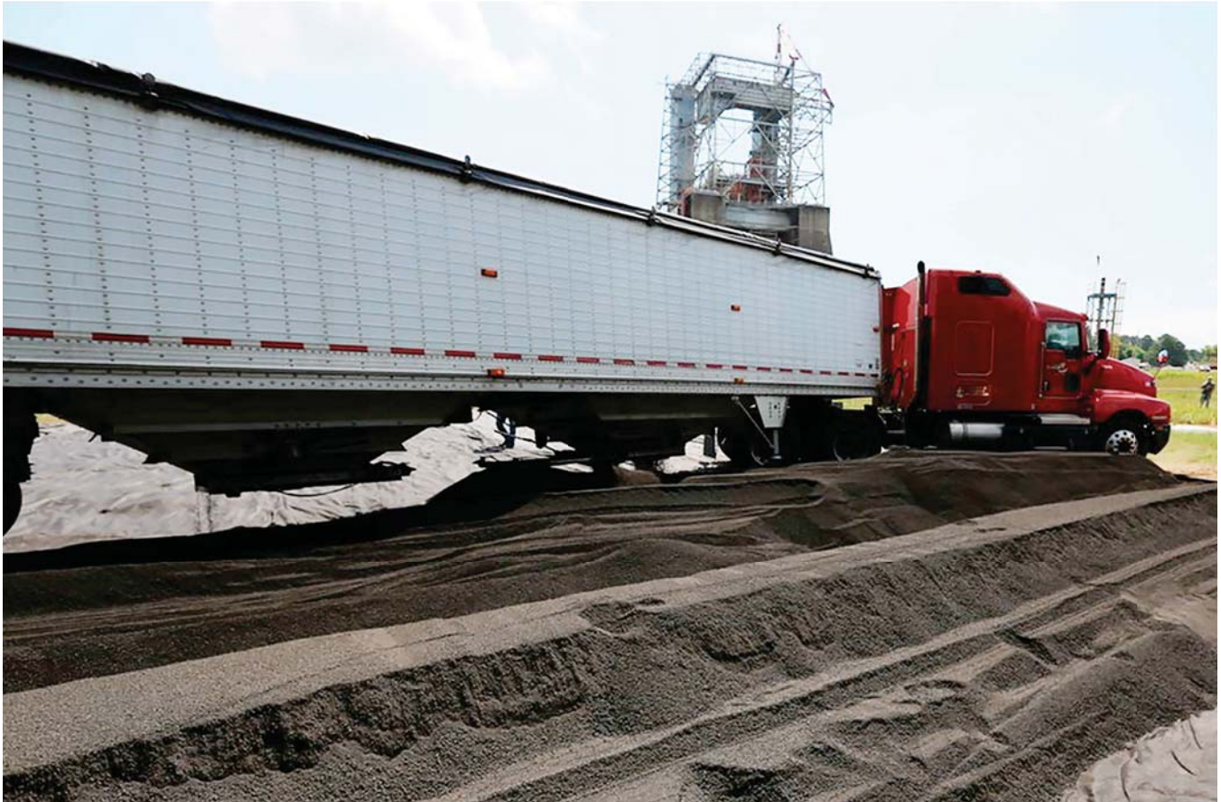
Figure 6. Belly dump trailer unloading volcanic cinder for the MSFC Lunar Surface Testbed.
