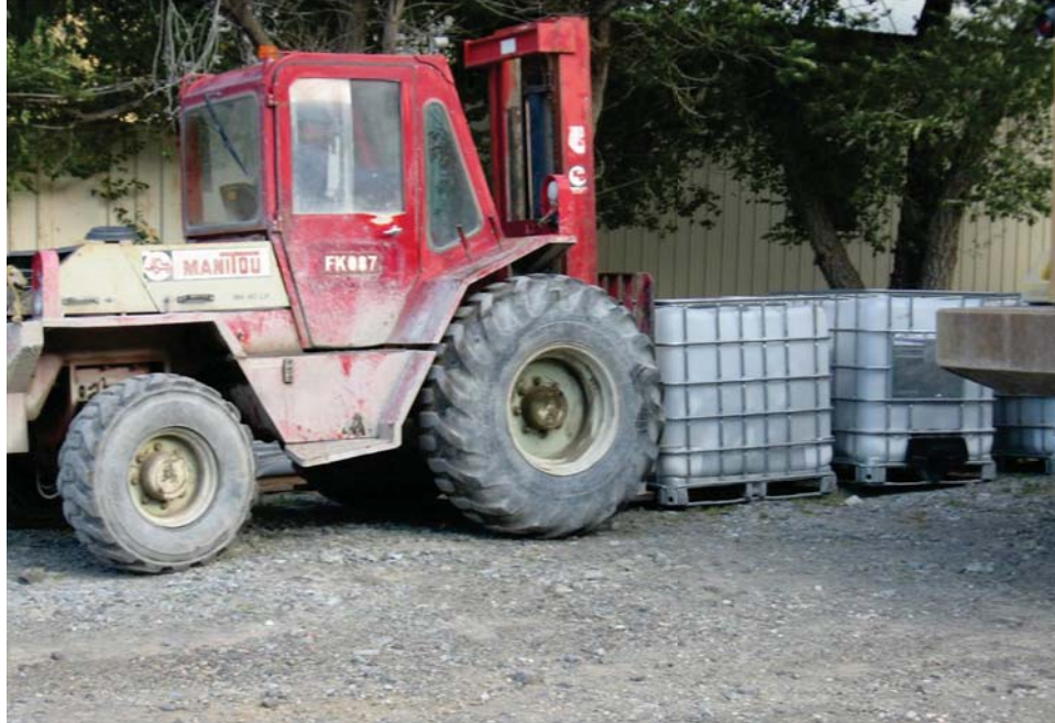
Figure 4. IBCs being moved by forklift. Photograph taken by author at the Stillwater Mine, Nye, MT; used with permission of mining company.
