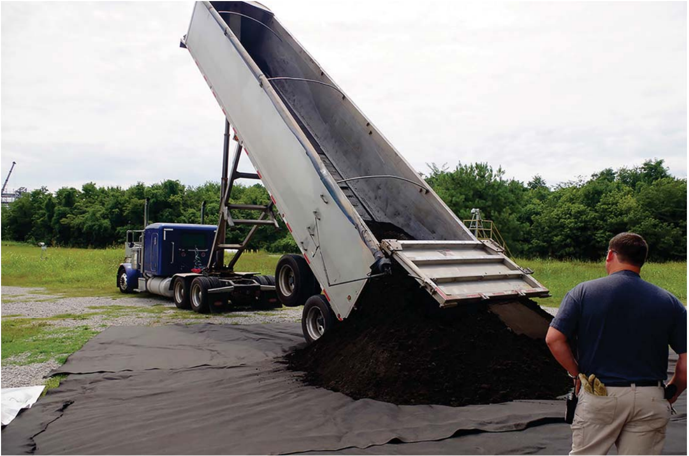
Figure 7. Belly dump trailer unloading volcanic ash for the MSFC Lunar Surface Testbed.
