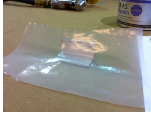
Figure 6.—Plastic film was used with some materials to allow the formation of a fillet with the Teflon rod.
