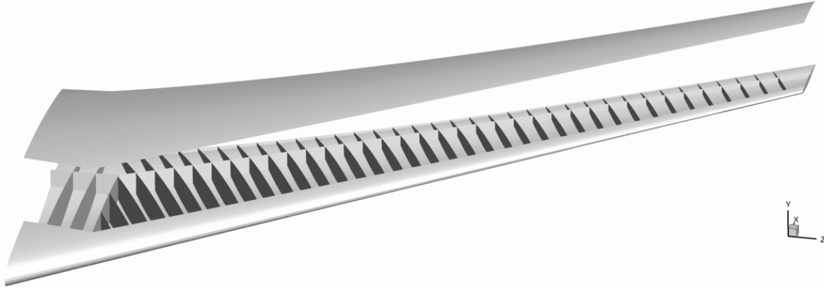
Figure 2: The QRM structural wing box
