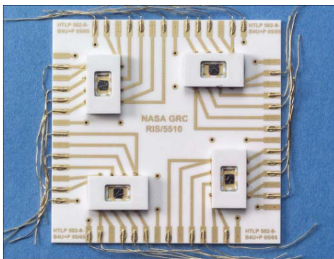
Figure 2: High temperature 96% alumina PCB with four packaged SiC devices [5]. PCB measures 2 inches by 2 inches.
