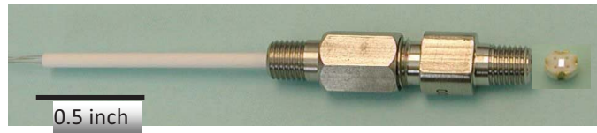
Figure 6: Spark-plug type package for high temperature SiC capacitive pressure sensor [11].
