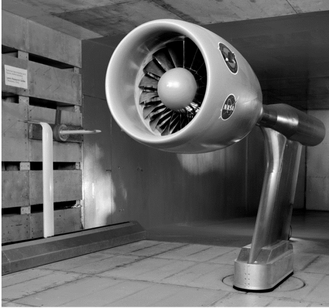
Figure 33.—Advanced Ducted Propulsor (ADP) fan test in 1995.
