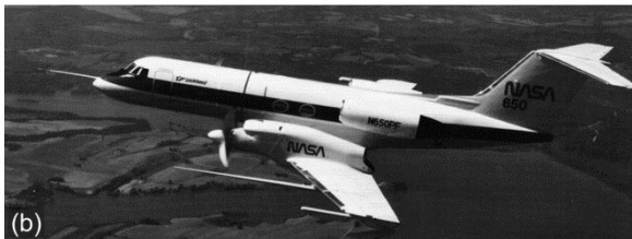
Figure 28.—Single-rotation propfan. (a) SR-7A in the 9×15 LSWT. (b) Propfan Test Assessment (PTA) aircraft with wing-mounted propfan.
