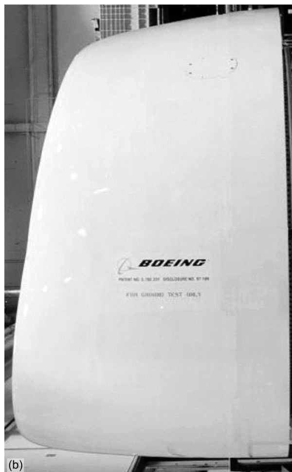
Figure 39.—PW4098 engine test. (a) Pratt & Whitney (P&W) C11 test stand. (b) Boeing scarf inlet.
