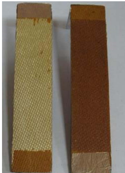
Figure 5. Example of "adhesional" failure of an exposed adhesive bonded joint specimen during laboratory testing.
