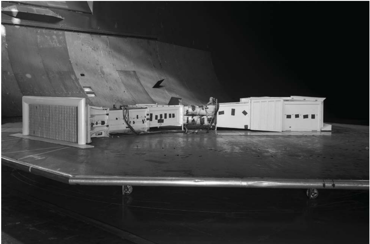
Figure 2. 1/50th-scale model of the NFAC 40 x 80 x 120 in the 40- by 80-Foot Wind Tunnel for testing in 1976.
