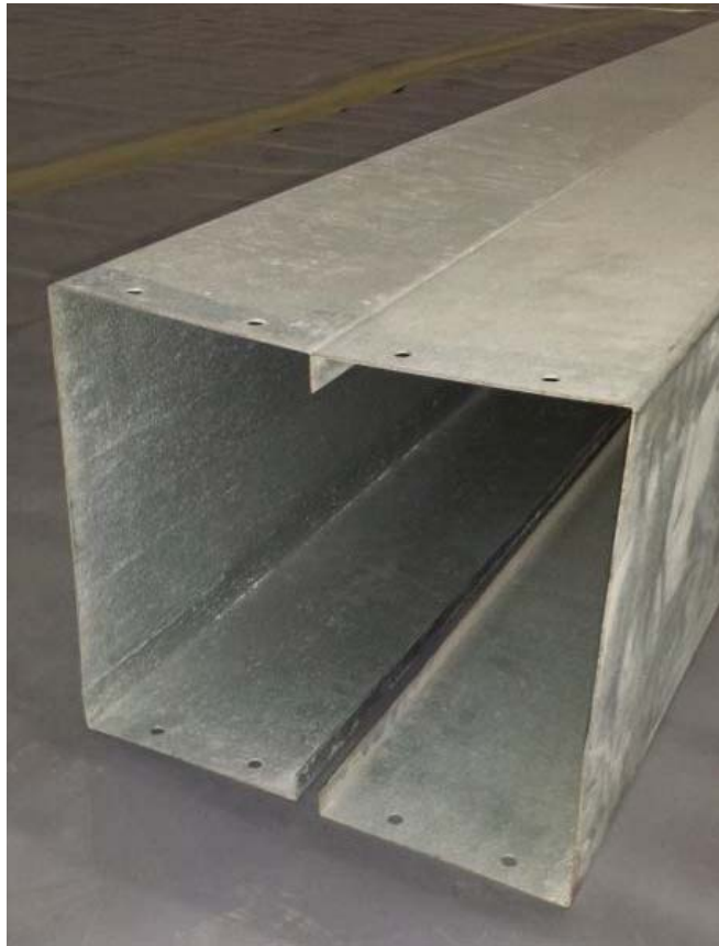
Figure 12. Box beam used to simulate blockage in front of inlet.
