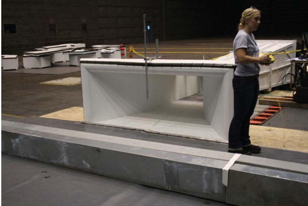
Figure B5. Blockage 4 feet ahead of inlet (runs 332, 333).
