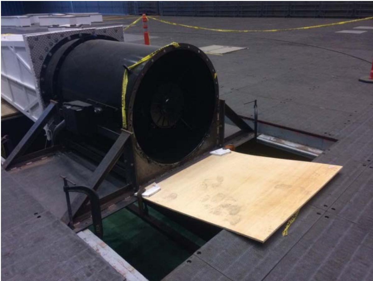
Figure 5. D/47 vane axial fan from Chicago Blower Corporation attached to rear of 1/50th-scale model.
