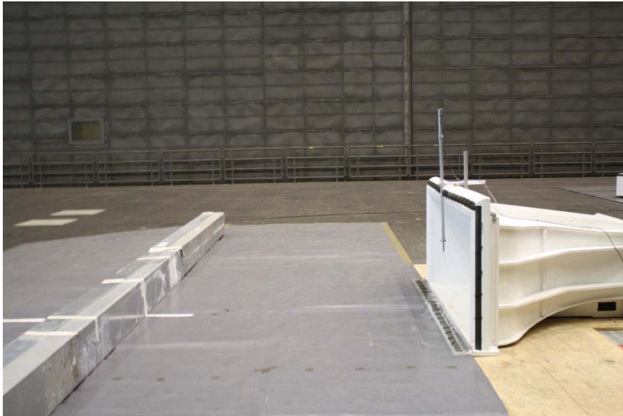
Figure B14. Box-beam 8 feet upwind from the inlet (runs 348, 349).
