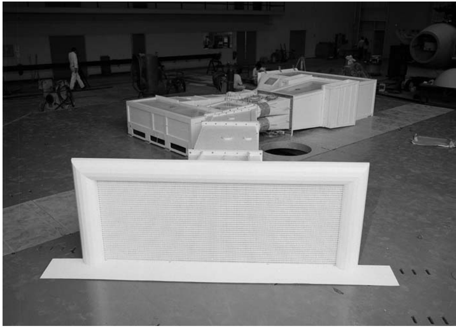
Figure 1. 1/50th-scale model of the NFAC 40 x 80 x 120 as tested in 1976.
