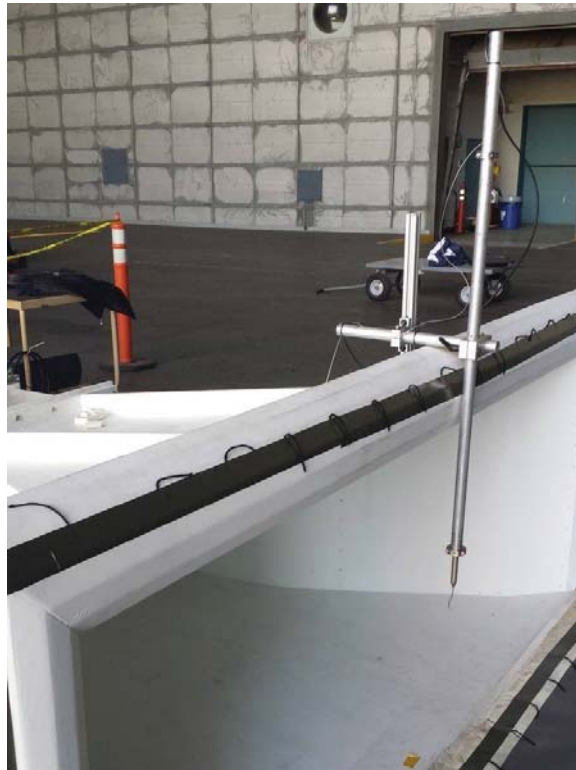
Figure 8. Cobra probe mounted at centerline of 1/50th-scale model inlet.
