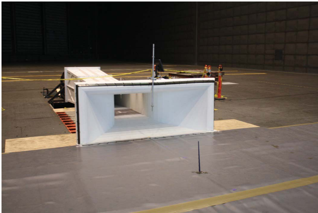
Figure E6. Inlet with weather tower. Note: the weather tower is slightly offset from the inlet centerline.
