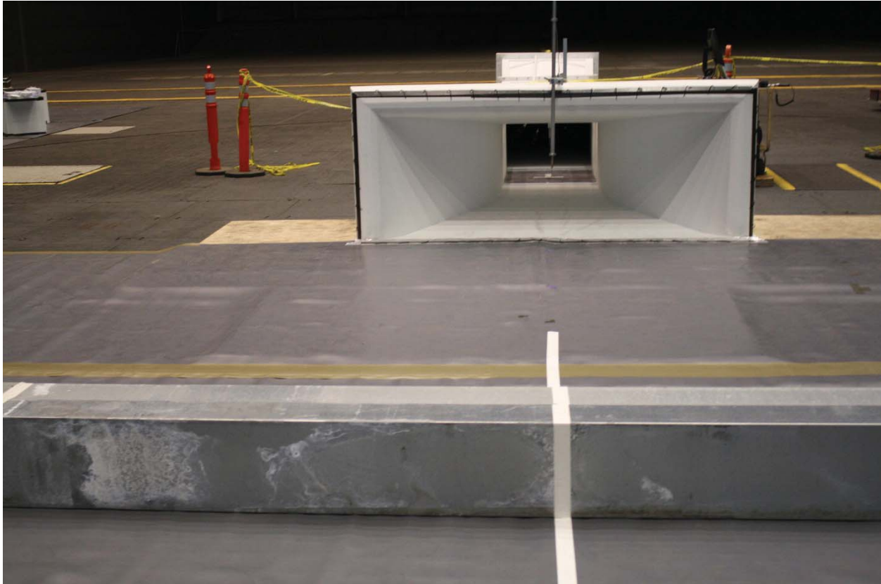
Figure B8. Blockage 12 feet upwind from inlet (runs 336, 337).
