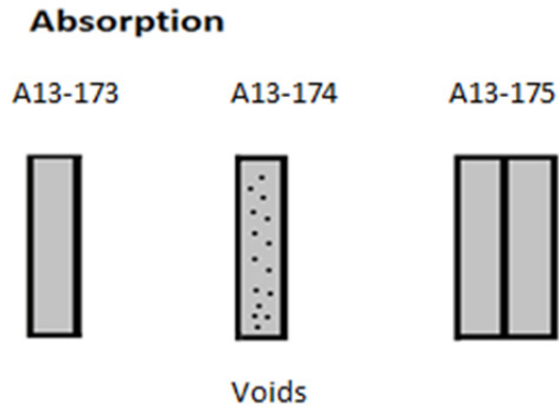
Figure 1.—Cross-sectional views of NEMFAT absorption test configurations.
