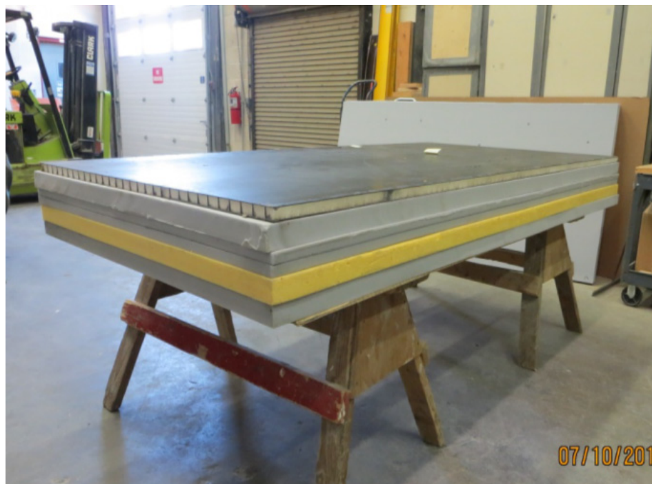
Figure 9.—The 8-in.-thick combination foam treatment (TL13-144) (top to bottom layers: FRF panel, 2-in. ML foam, 2-in. ML foam with center mass barrier, 2-in. ML UL foam, 2-in. ML foam).
