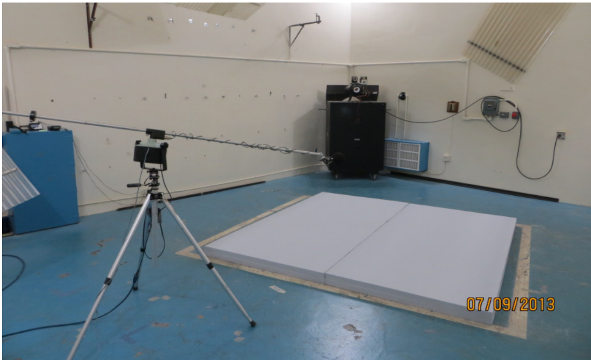
Figure 2.—RAL’s absorption test setup (4-in.-thick ML foam, ASTM-C423 reverberation room method).
