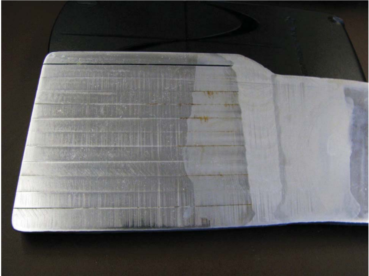
Figure 2 - Cross section of the head to shell weld of the A. O. Smith pressure vessel MV50466-8 (section provided by SwRI)
