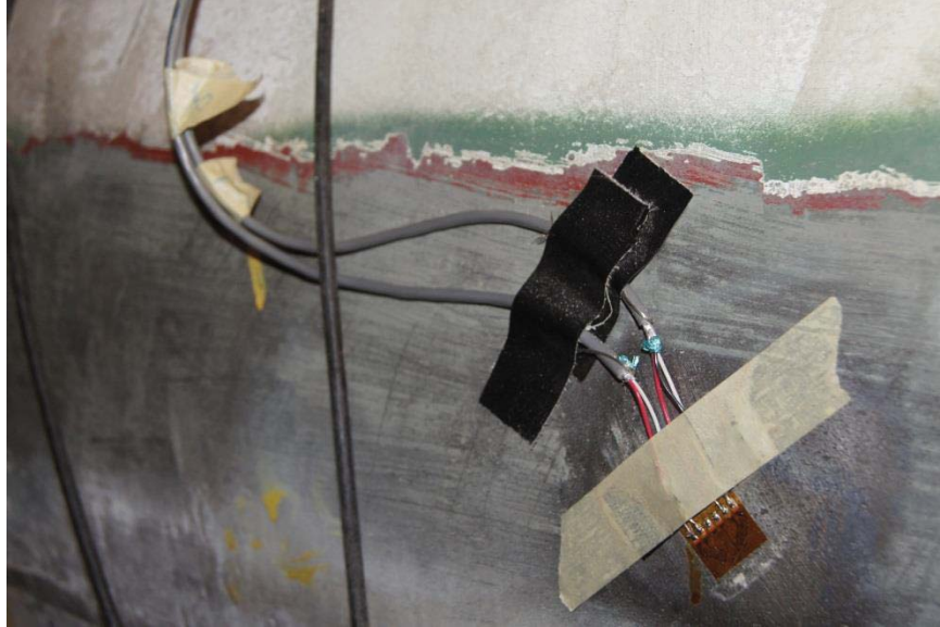
Figure 9 - Strain gages mounted at the center of the vessel
