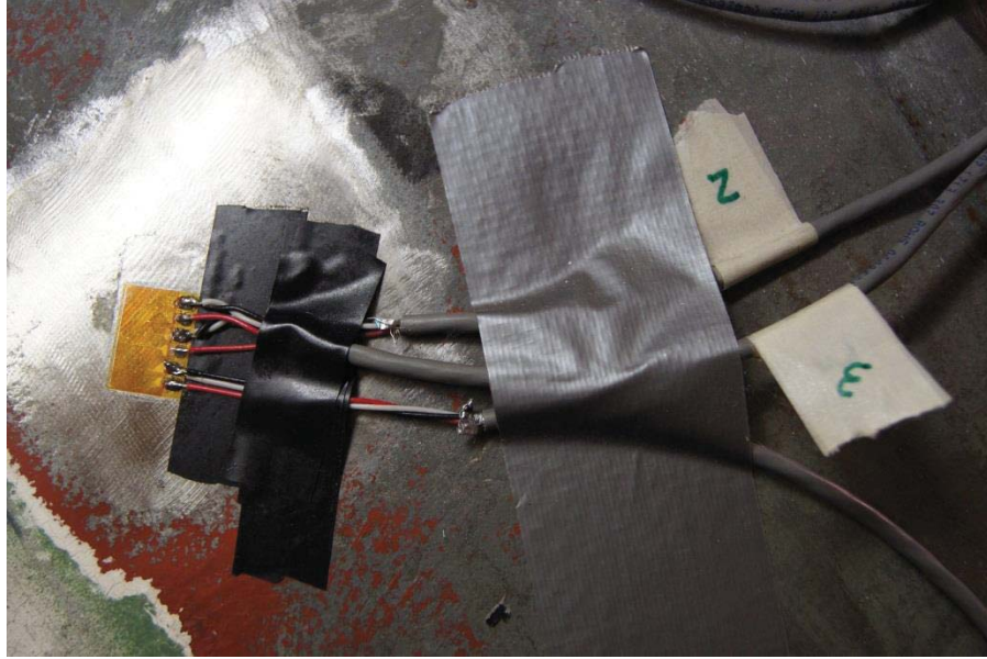
Figure 7 - Strain gage mounted on the vessel head
