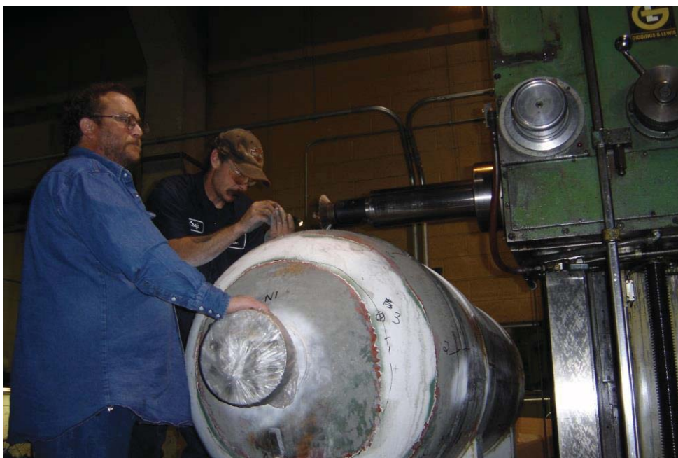
Figure 4 - Milling of the flaws into the vessel.
