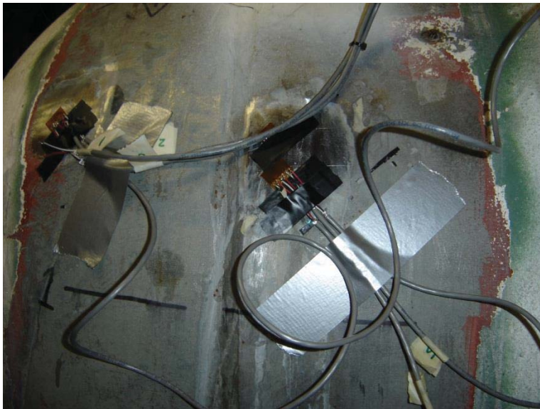
Figure 6 - Strain gages mounted on the head and near the head-to-shell weld of the vessel
