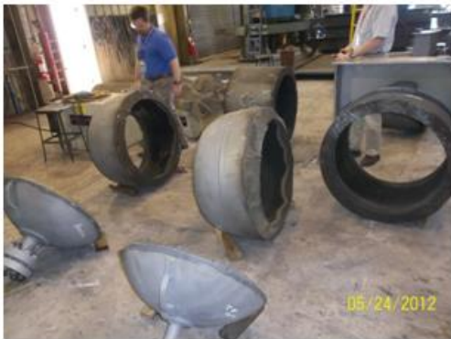
Figure 2-3. Photos of Sectioned Pressure Vessel
