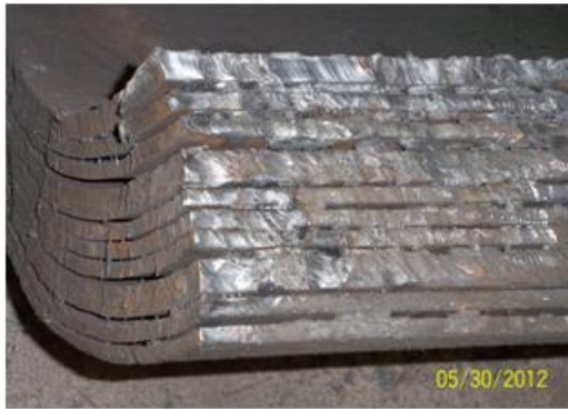
Figure 2-3. Photos of Sectioned Pressure Vessel
