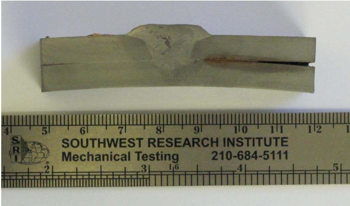
Figure 2-3. Outer Layer Seam Weld and Penetration into Inner Layer
