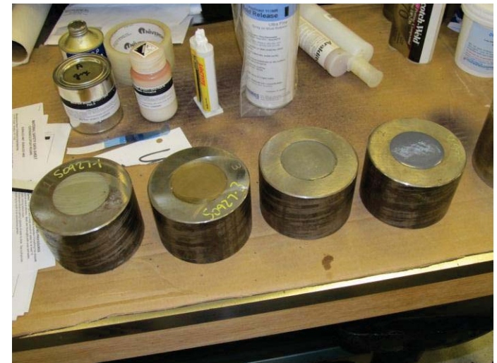
Seal Material Samples for Environmental Load Testing
