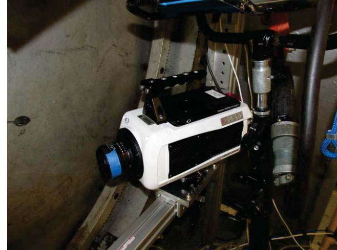
Phantom V611 installed at the 10x10 for the ExoMars Tests
