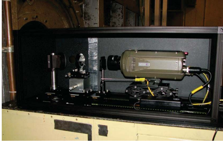
Phantom V310 Installed in Schlieren System
