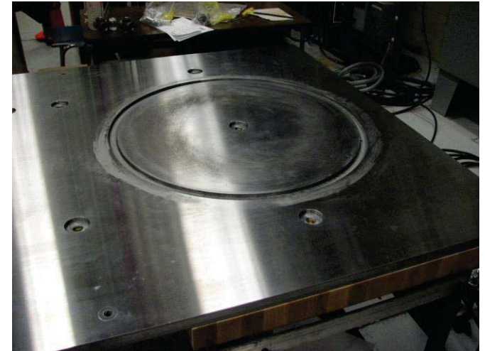
Steel Schlieren Window Installation Table
