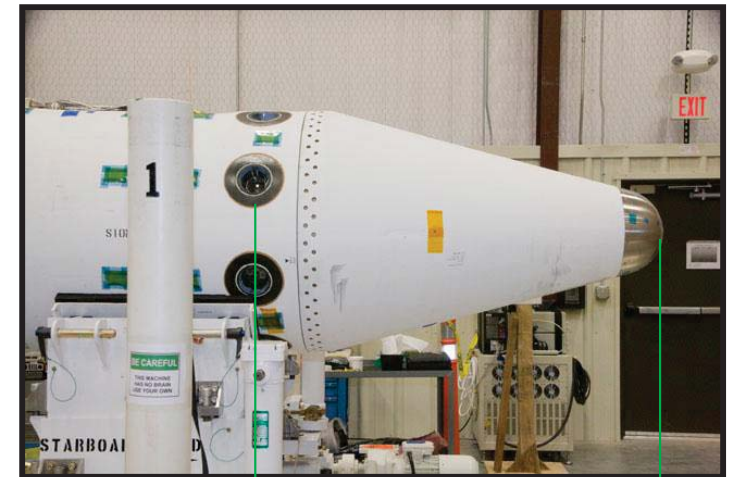
~ 48" Distance of FADS ports from ACM nozzles
