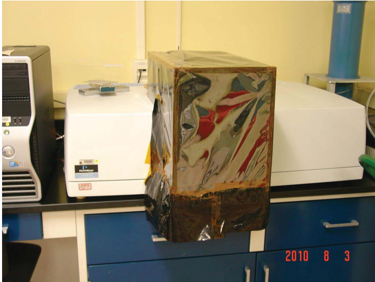
Figure 9. Black Cover used for more accurate calibration of instrument and to set baselines (normal cover would not allow all 5 point measurements to be covered)
