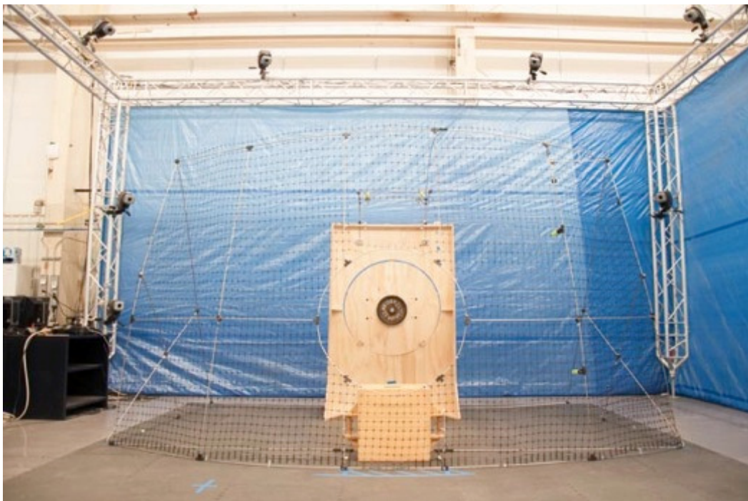
B-5. Phase 2 Mockup of Launch Vehicle Stage Adapter Wall Section with Hatch Opening, Connectors Requiring Tool Manipulation (right side) and Simulated LRU Equipment Shelf Attached to Plywood Structure
