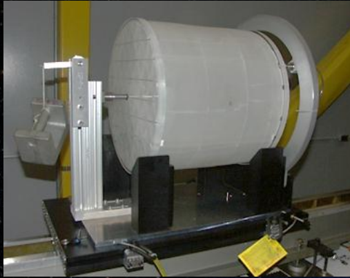
Subscale Deep Core Mirror Static Load Testing
