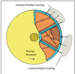
Figure 3. Diagram of typical forced radial cooling of foil bearings.
