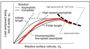
Figure 1. Operating regimes of gas foil thrust bearings demonstrating the low speed approximation, high speed asymptote, and high speed performance drop-off.
