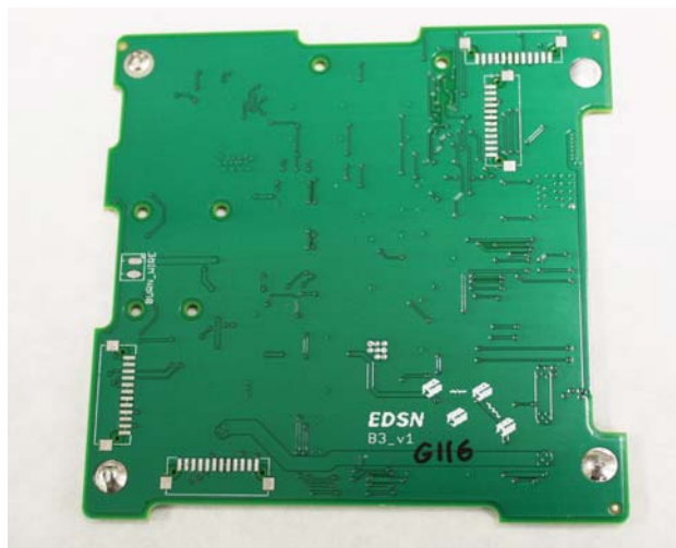
Figure 3. Uncoated EDSN G116 green circuit board, numbered side.
