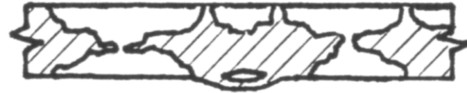
Damage Class C4: Perforation
