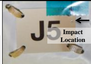
MPLM grapple fixture coating spall dia. = 0.6 mm
