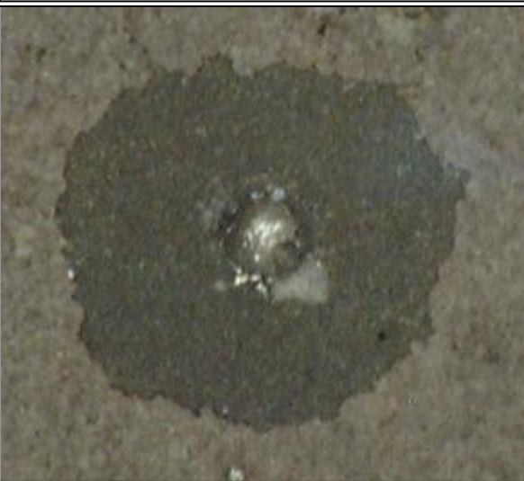
MPLM grapple fixture coating spall dia. = 0.6 mm
