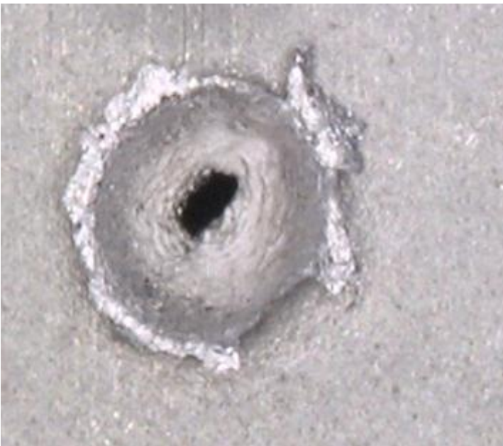
MPLM perforation A3 corner panel (exterior)
