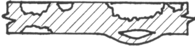
Damage Class C3: Detached spall
