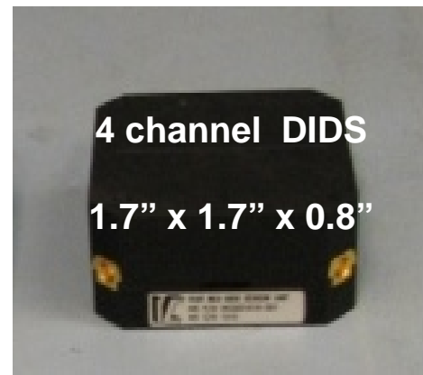
Distributed impact detection system (DIDS)
