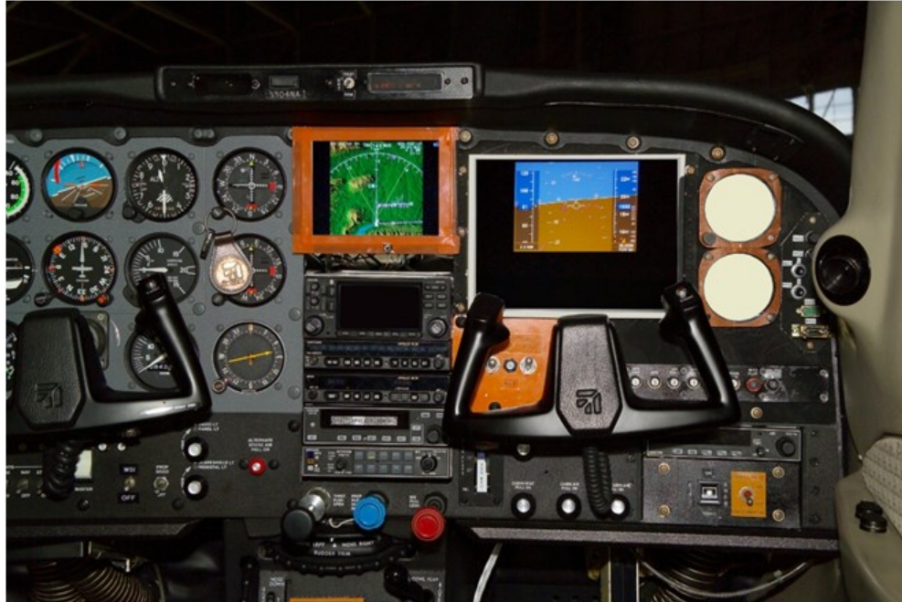
Figure 4: Pathway-Based Guidance Display Concept
