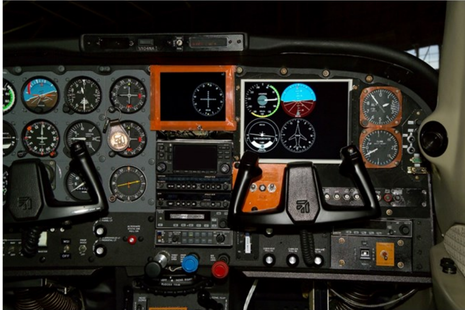
Figure 2: Baseline Round-Dial Display Concept
