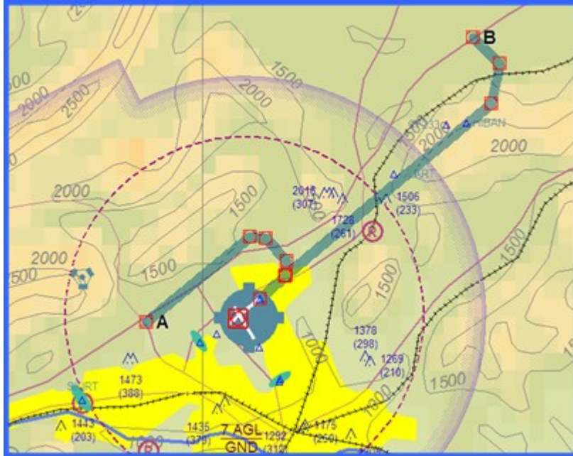
Figure 8a: VFR Sectional Map View with Approaches Overlaid
