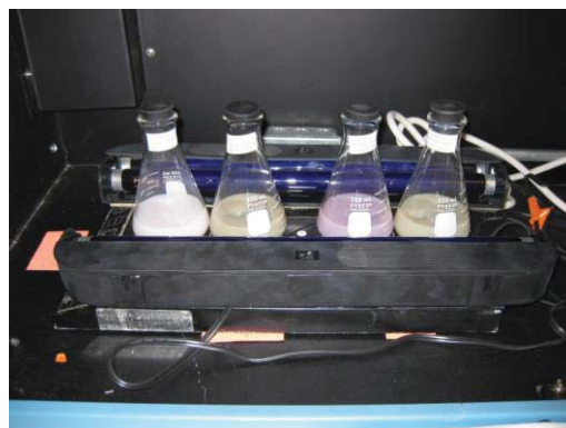
Figure 2: Photodeposition preparation method for quantum dot formation on TiO 2 .
