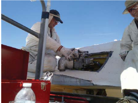
Figure 4. Removing an EPU from a retired F-16 at Davis-Monthan AFB.
